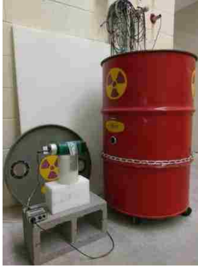
Fig. 58. Detector set-up for PuBe measurements
