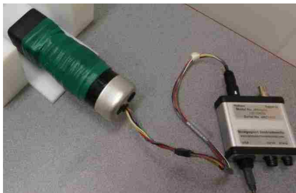
Fig. 57. Detector assembly for PSD testing of EJ-299-33A
