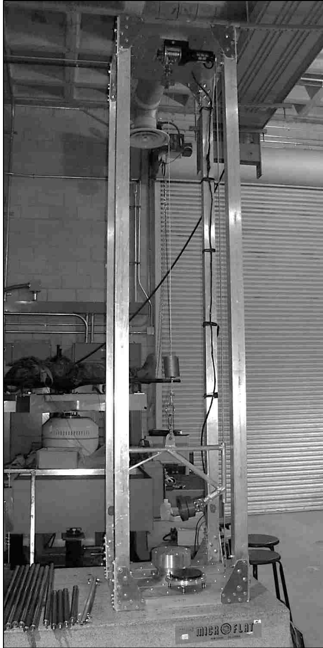
Figure 9: Test Frame in Drop Tower Configuration [1]
