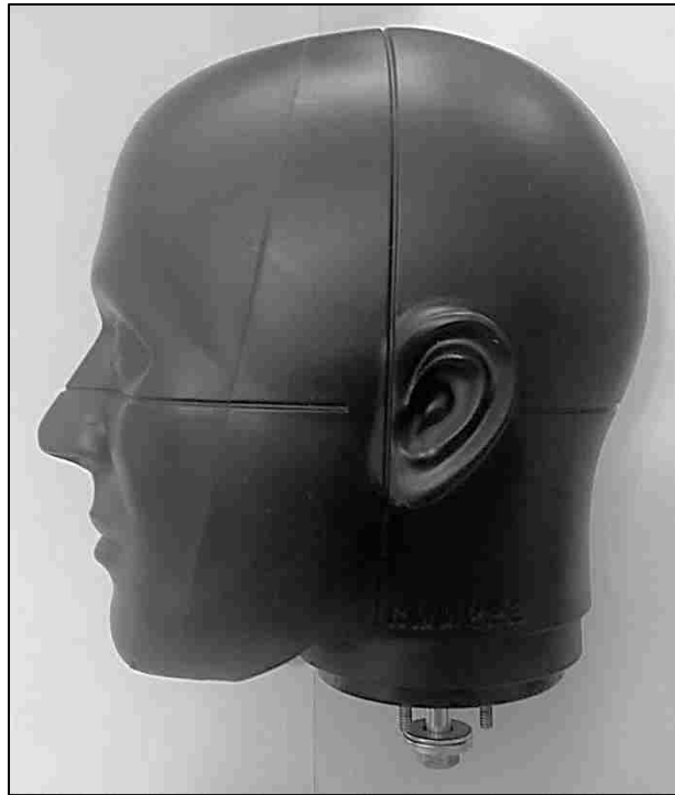
Figure 7: Southern Impact Research NOCSAE Headform Size Medium
