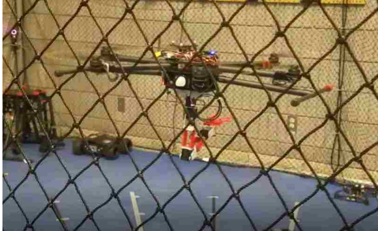
Figure 6.39. Closed-loop parallel hexrotor aerial manipulation test.
