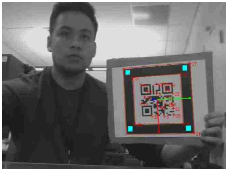
Figure 6.37. QR code detection and pose estimation of the target.
