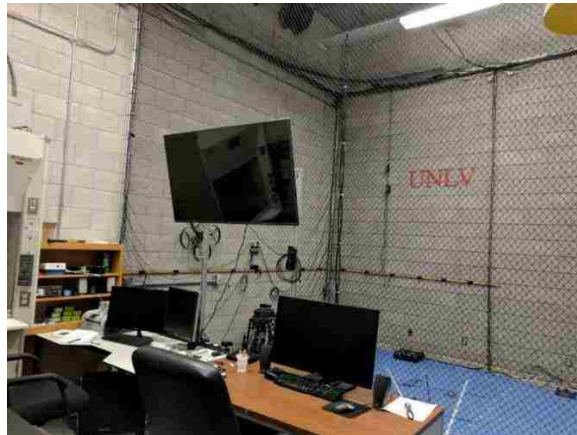
Figure 6.1. UNLV indoor flight volume equipped with an Optitrack motion capture system.
