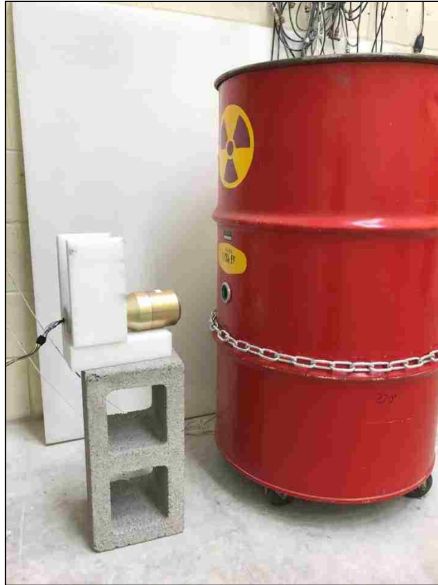
Figure 43. Measurement configuration of CLYC-7 scintillator with a PuBe source at the UNLV Nuclear Engineering Laboratory
