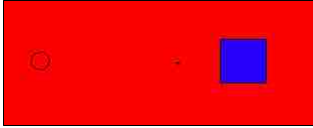
Figure 35. MCNP model of 2 inch-by-2 inch CLYC-7 scintillator with source; the blue square is a CLYC scintillator, the red circle and square surrounding CLYC is air, the red-filled circle contains 0.0253 eV or 3.5 MeV point source.
