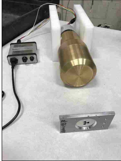
Figure 42. Measurement configuration of CLYC-7 scintillator with the ^{137}\text{Cs} photon source at the UNLV Nuclear Engineering Laboratory
