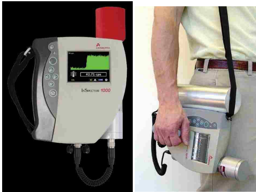
Figure 20. The Canberra InSpector™ 1000 Digital Handheld Multichannel Analyzer with optional NaI:Tl gamma-ray probe (left) and with optional neutron probe (right) [24]
