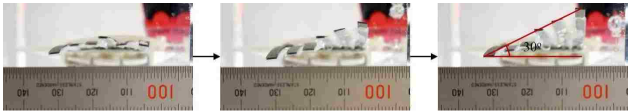
Figure 6.13 Twisting deformation of the soft fin.
