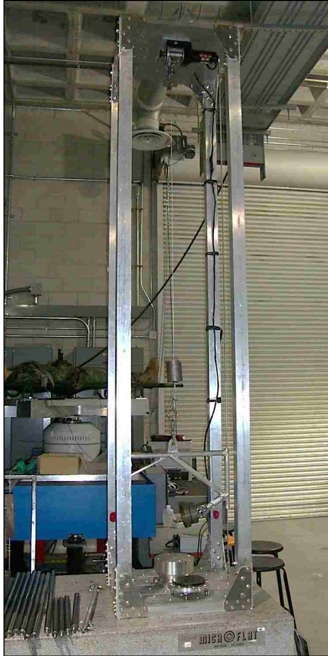
Figure 4-2: Full Length View of Hybrid Impact Tower
