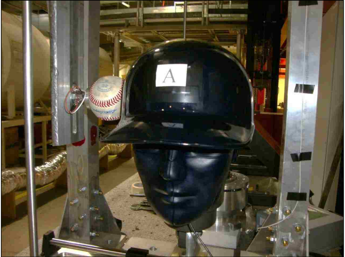
Figure 4-5: Free End of Pendulum with Load Cell & baseball Adapter
