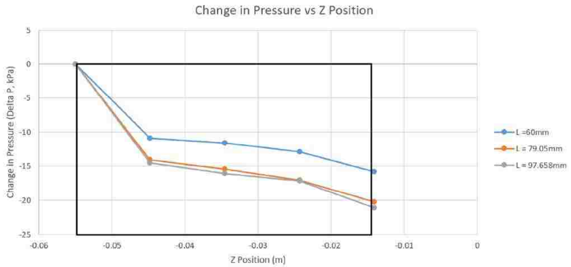
Figure 26 Averaged pressure across different Z position slices over fluid domains with different total lengths, highlighted box denotes spacer location
