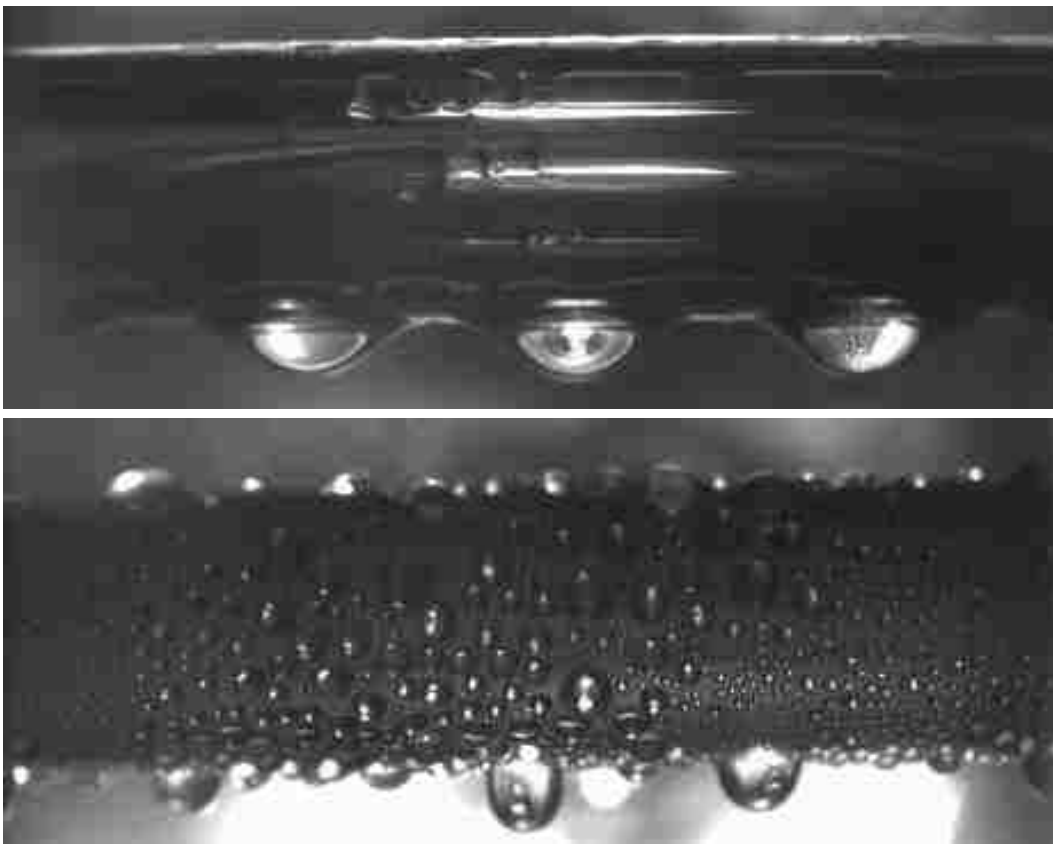
Figure 1. Filmwise and Dropwise Condensation on Horizontal Tube
