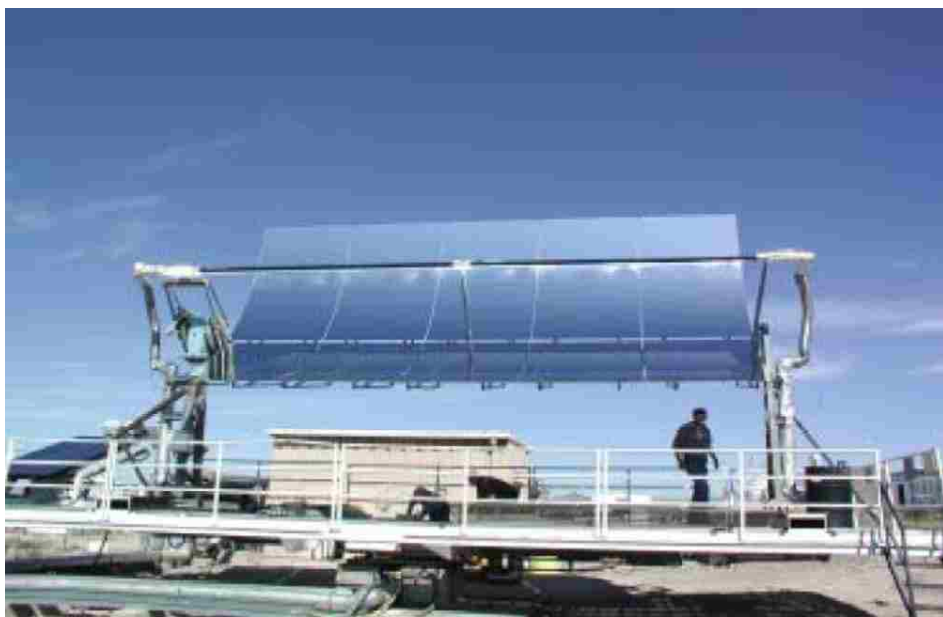
Figure 33 LS-2 collector test at Sandia National Laboratory, USA [37]
