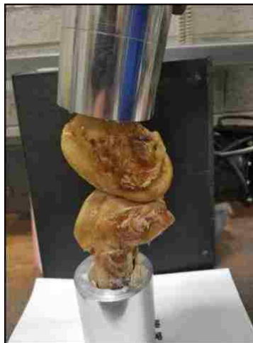
Figure 1-4: KTA Joint Placement Using Pig Femurs. 3
