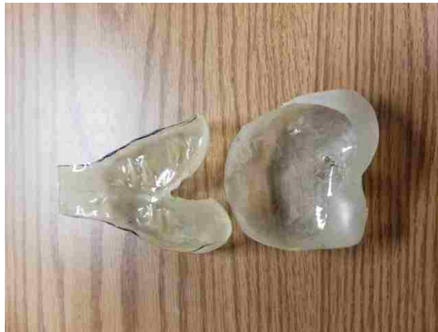
Figure 1-2: Chronoflex Implant Created Manually by Brushing Layers
