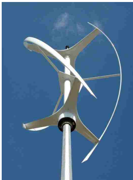
Figure 4: Darrieus turbine example (“Sky Harvest to acquire vertical axis wind turbine technology and manufacturing facilities,” 2013)
