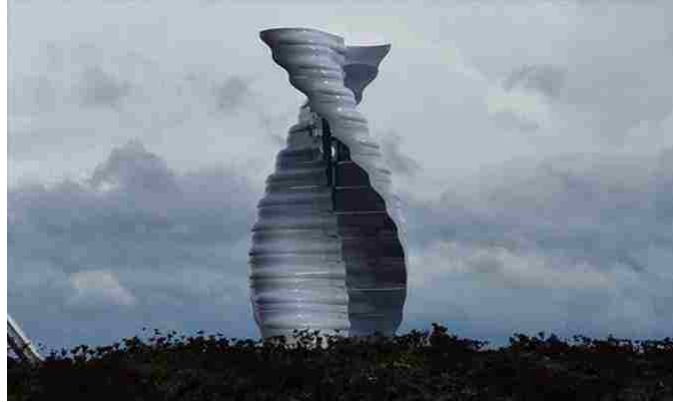
Figure 3: Savonius rotor example (“The Benefits of the Helix Wind Turbine - UAT Group,” n.d.)
