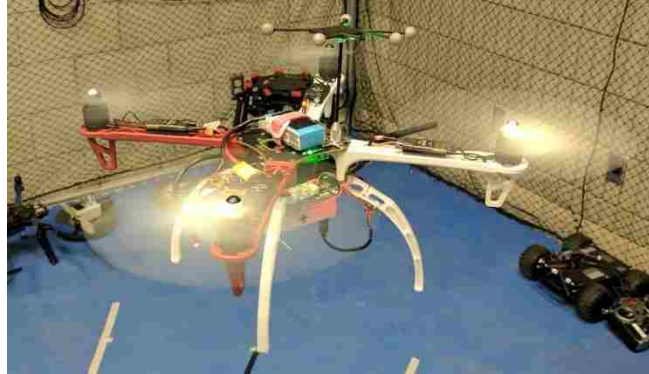
Figure 31: DJI Flamewheel F450 with onboard Odroid-UX4 SBC and Optitrack ridged body markers positioned on the GPS Stand.
