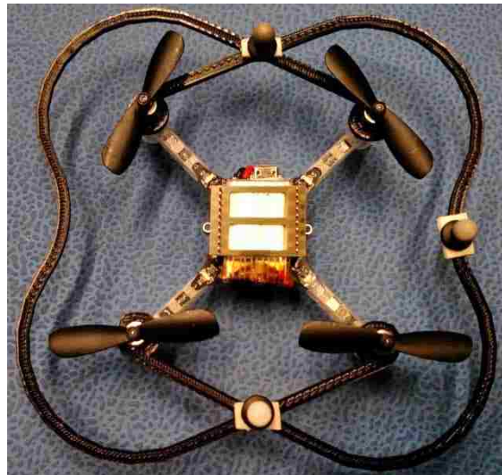
Figure 30: Crazyflie 2.0 with 3D printed propeller guards. The reflective markers for motion capture are placed along the propeller guard in a formation unique to each UAS.
