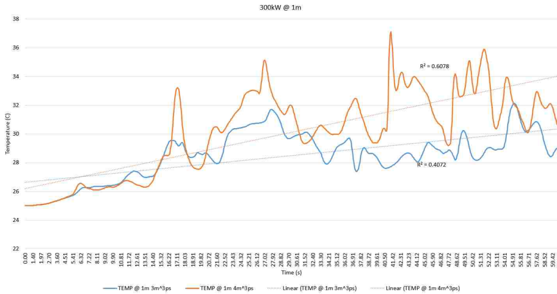
FIGURE 4.10. Exhaust vent: 3 - 4 m 3 /s, thermocouples at 1m, cor=0.736384
