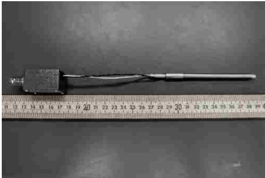
Figure 5.4: Helium-3 proportional counter [6].
