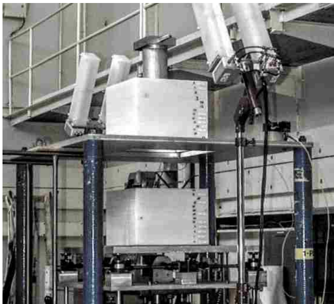
Figure 5.2: The Planet vertical lift assembly (shown here with the Class Foils experiment) [4].
