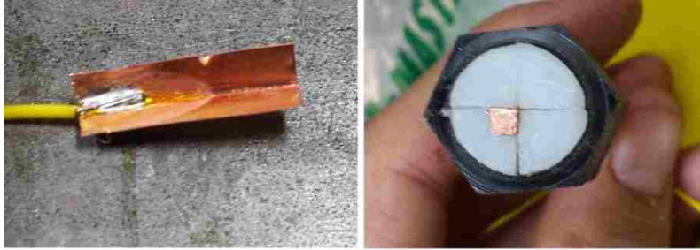
Figure 3.12: Wire soldered to copper foil ( left ), and copper foil attached to nylon collet for one corner of the collet ( right )
