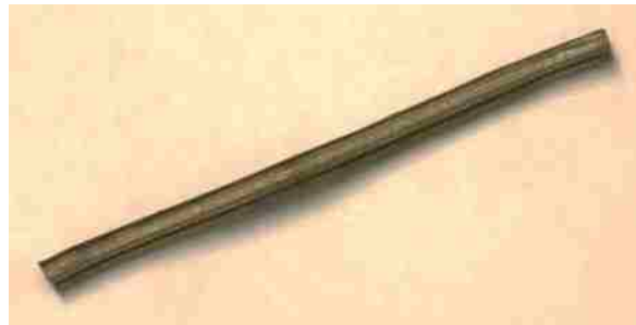
Figure 3.11: Photograph of a tube-shaped IPMC sample
