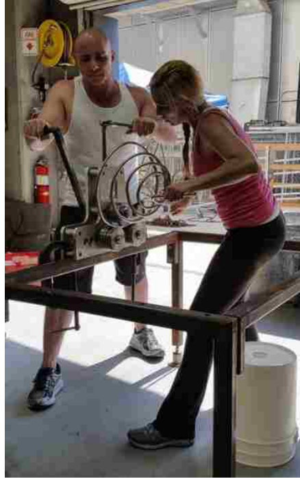
Figure 11. Component Fabrication using the UNLV Adjustable Radii Tube Bender Tool
