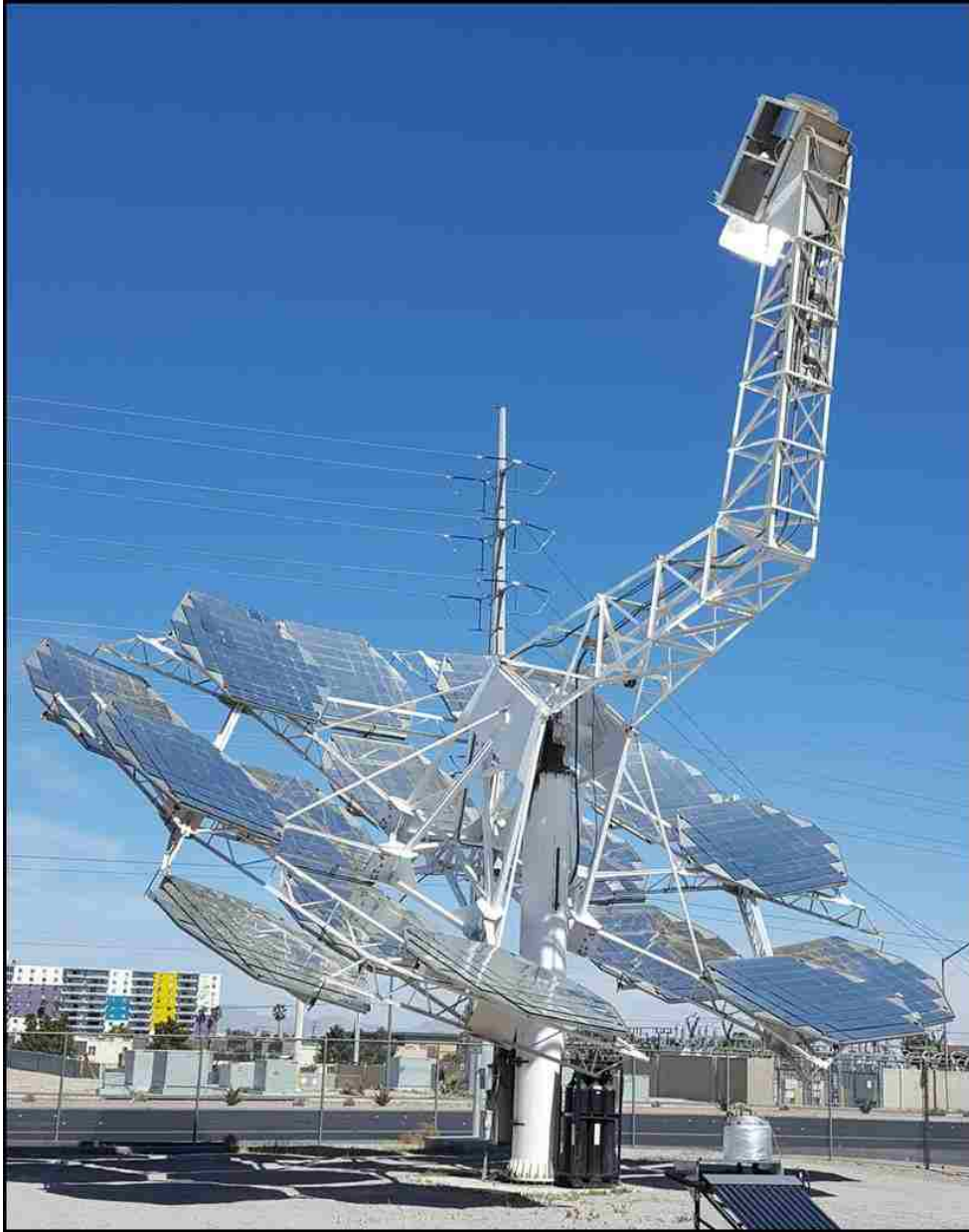
Figure 2. SAIC Dish On-Sun Testing
