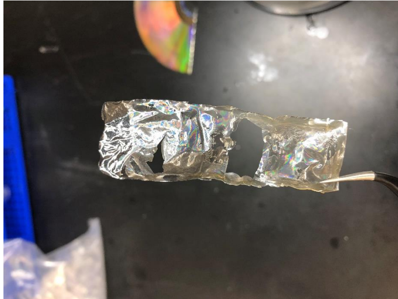
Figure 7: Nanoimprinted silk film with significant dissolved sections.
