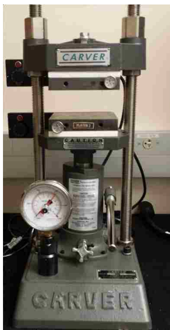
Figure 2.12: Carver, Inc. (Model # 3851-0) heated press used to press the mold halves together
