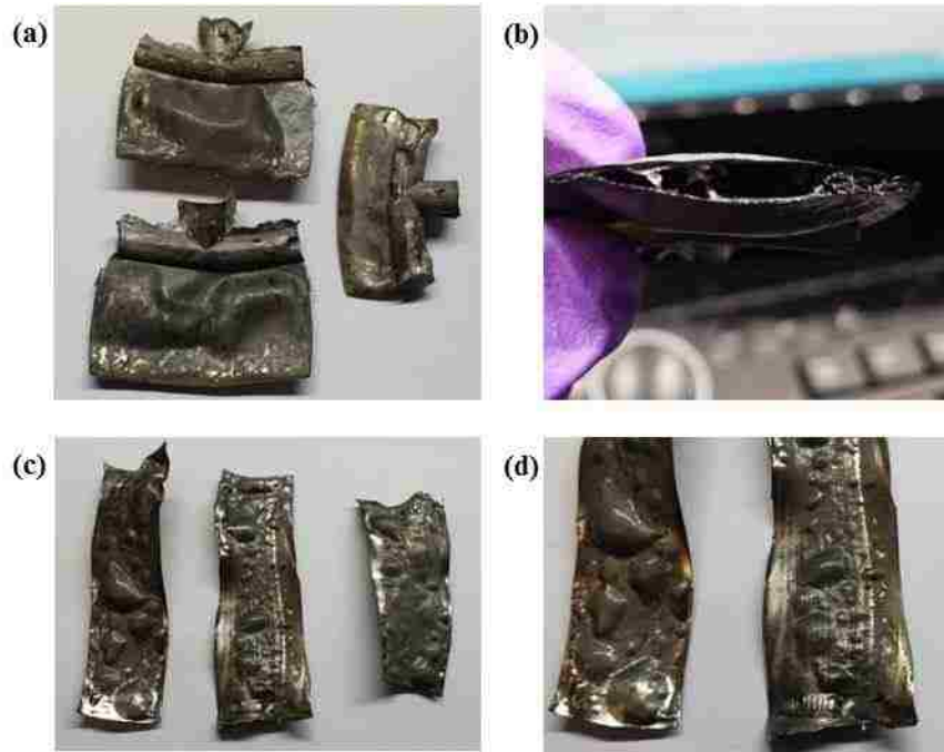
Figure B.1: (a) Injection molded samples with air pockets, (b) injection molded sample inside air pocket, (c) extruded samples with air pockets, (d) close up of extruded samples
