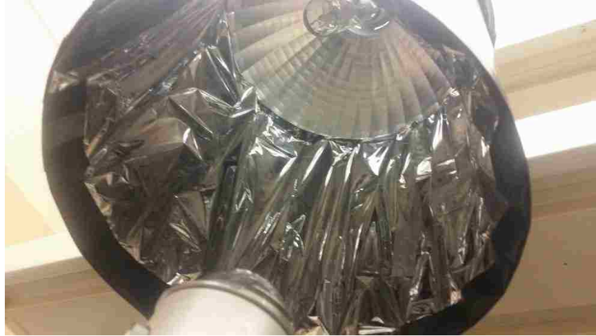
Figure 19: Aluminum hollow cylinder with Mylar coating around inner surface
