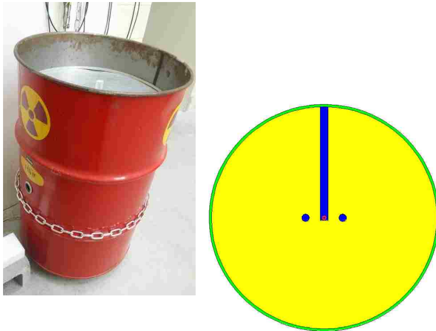
Figure 4.11 Pu-Be drum (left) and MCNP cross sectional model (right)
