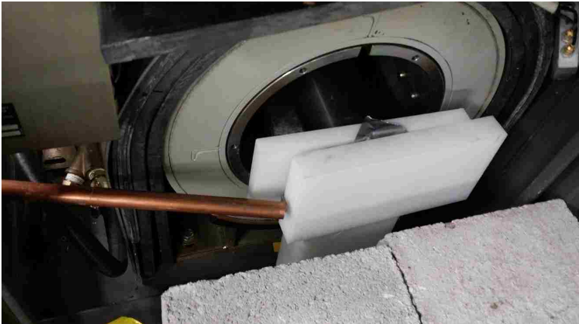
Figure 5.12 Irradiation setup for the Varian M6 photoneutron source.
