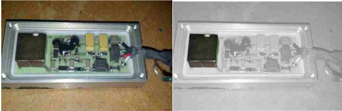
Figure 5.6 CZT detector with preamp electronics (left) and active 10mmx10mm CZT face (left highlighted).
