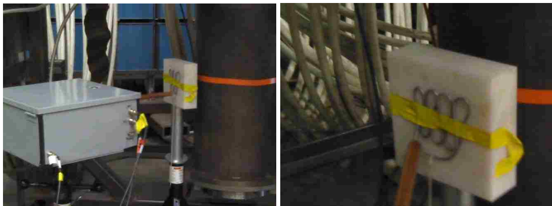
Figure 5.8 Irradiation setup with pump and detector, transport line to moderating material and DPF neutron source (left) and close up of transport tubing on moderator
