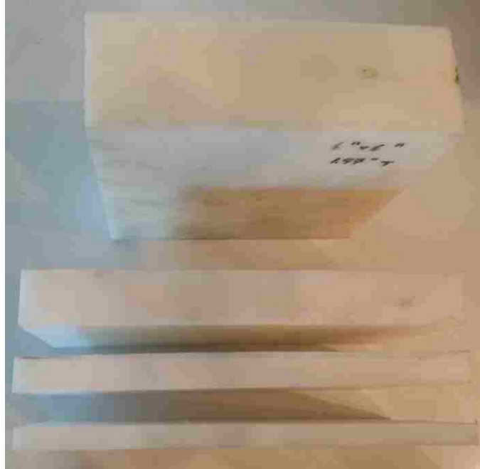
Figure 4.5. Physical polyethylene pieces used for DPF and Varian M6 moderating and reflectors.
