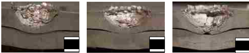
Figure 3.6: Deformation vs. impact velocity for 2-layer plates at velocities of (a) 5.6 km/s (b) 6.2 km/s (c) 6.7 km/s
