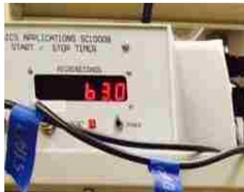
Figure 2.22: Digital readout of laser intervalometer
