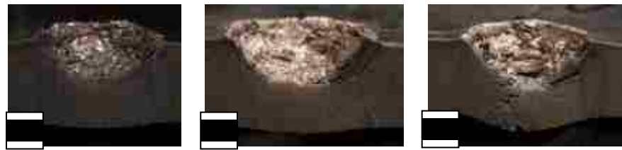
Figure 3.3: Deformation vs. impact velocity for AM 'B' 12.7 mm Ti plate at velocities of (a) 5.255 km/s, (b) 5.613 km/s, and (c) 6.08 km/s
