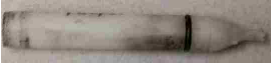
Figure 2.13: Used piston deformed into conical shape
