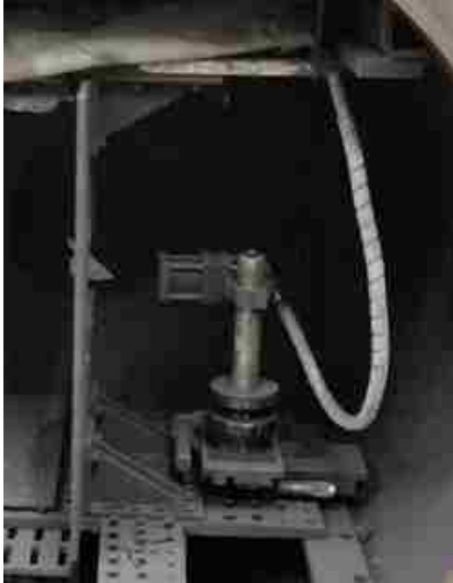
Figure 2.24: Linear mechanical transfer array
