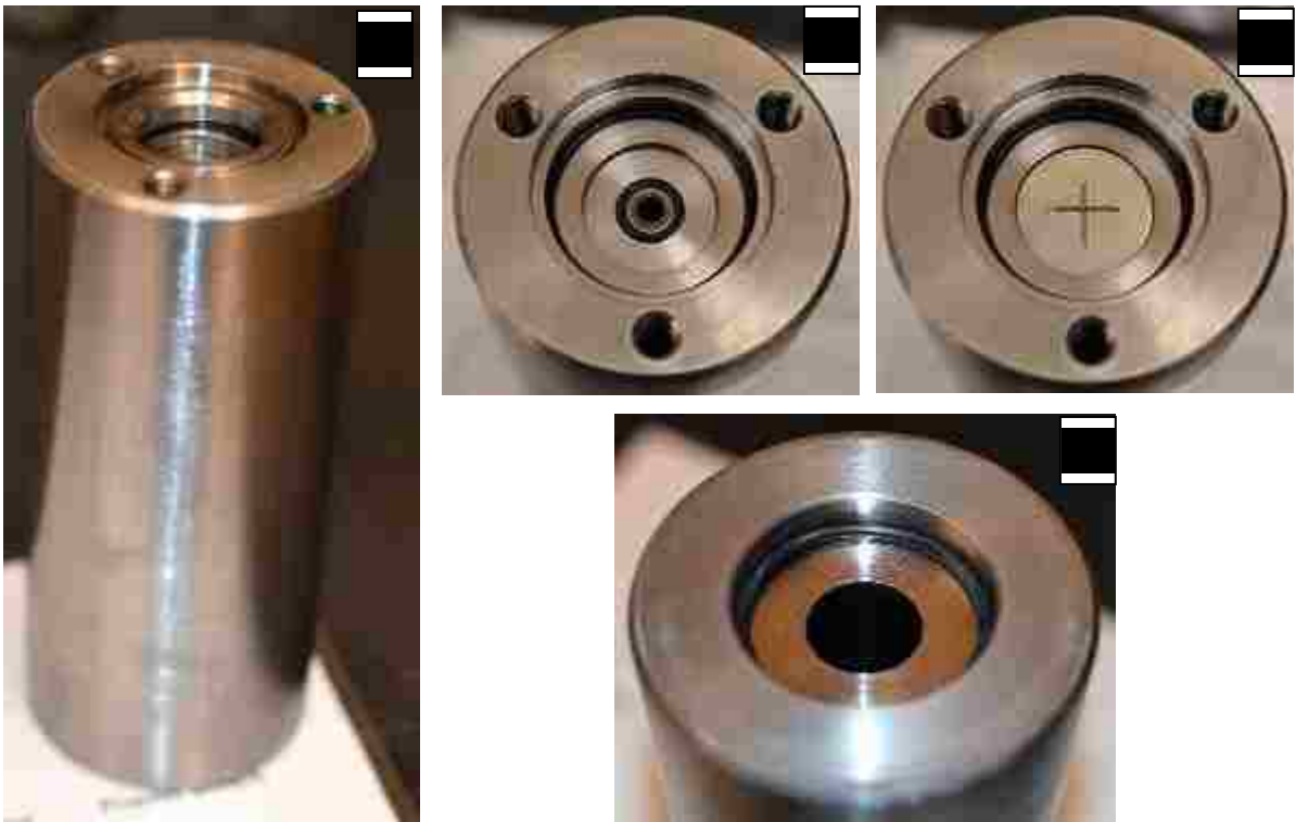
Figure 2.12: a) Central breech b) central breech launch tube end c) central breech with petal valve d) central breech pump tube end
