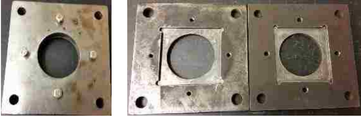
Figure 2.28: New target holder configuration
