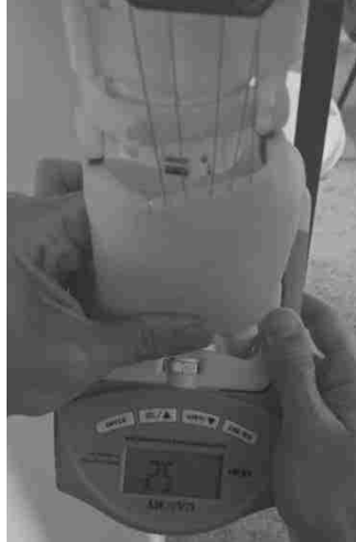
Figure 4.8: Upside Down Measurement of Grip Force using a Digital Dynamometer
