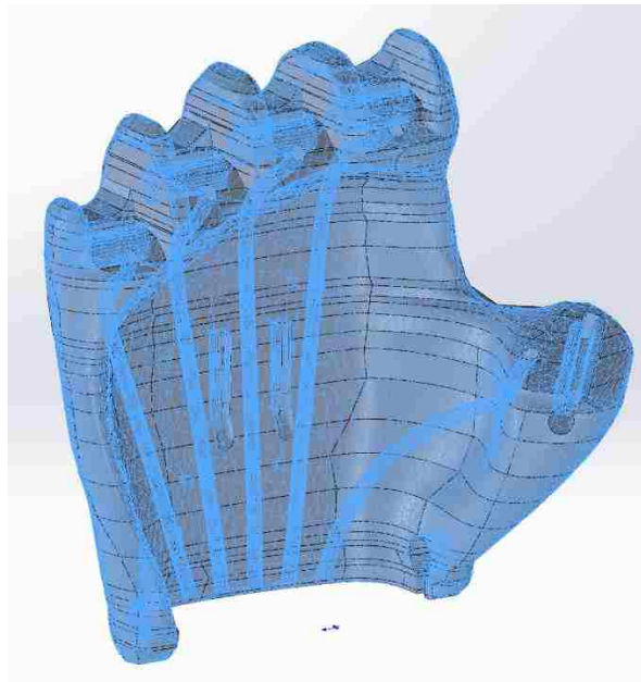
Figure 3.4: Flexy-Hand 2 Recreation in SOLIDWORKS ®
