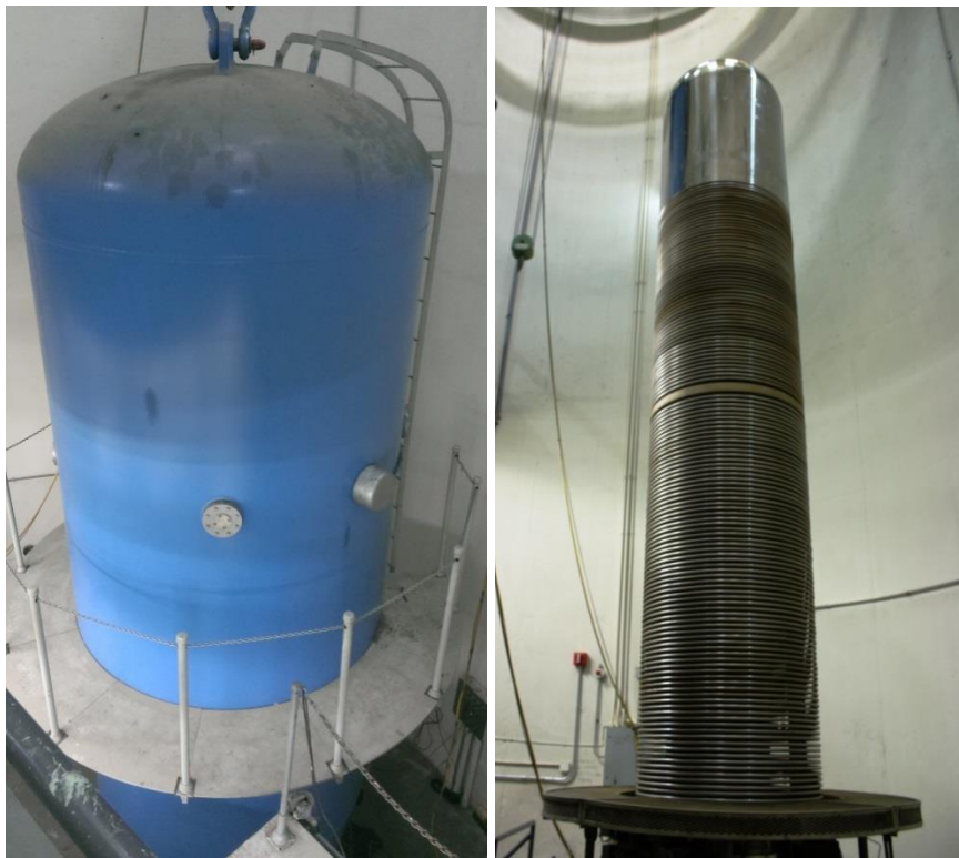
Figure 21: The University of Kentucky's particle accelerator with and without the protective covering that gives it its name.
