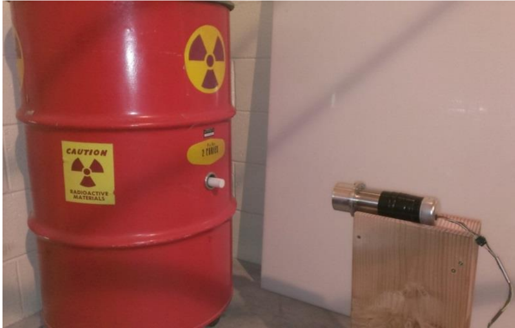
Figure 30: Experimental setup of the plutonium-beryllium source and EJ-299-33A detector.
