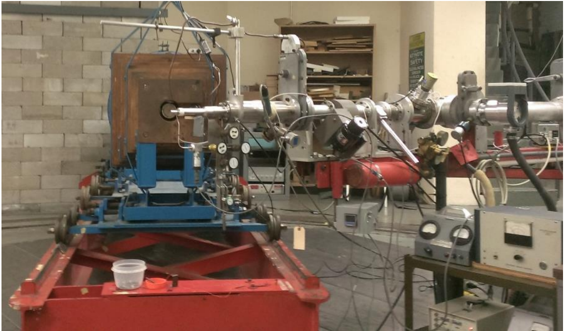
Figure 23: Measurement setup with beamline and detectors; 120^\circ orientation.
