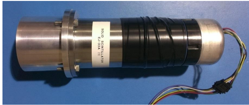
Figure 17: Assembled detector unit, with attached HVC base for signal output.
