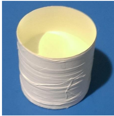
Figure 13: EJ-299-33A plastic scintillator used in detector design.
