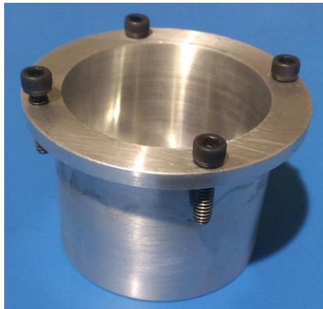
Figure 16: Aluminum cap for the scintillator material.
