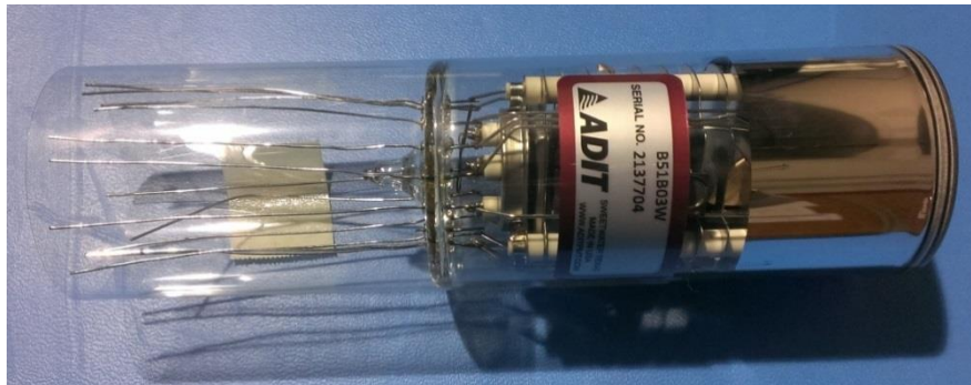
Figure 14: ADIT B51B03 PMT used in detector design.
