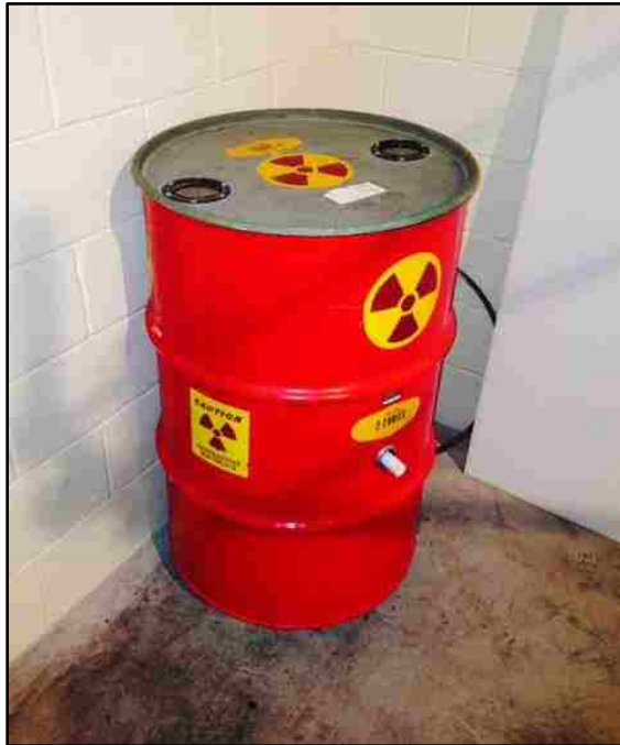
Figure 23 – Sealed PuBe neutron source in 55-gal steel drum utilized in this study
