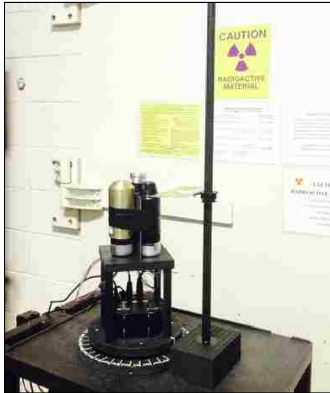
Figure 25 – CLYC detector system mounted to turntable, adjacent to latitudinal displacement source holder
