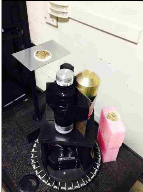
Figure 51 – Experimental setup for two source directional measurements
