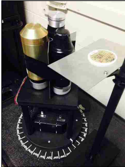
Figure 45 – ^{137}\text{Cs} gamma-ray directional measurements experimental setup, angled view
