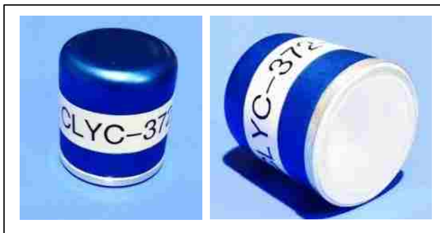
Figure 16 – Encapsulated 1-inch CLYC crystal used in experiments
