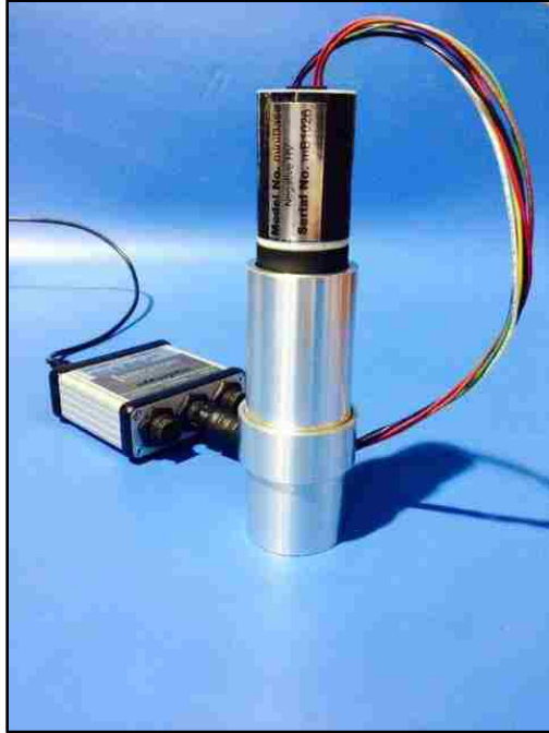
Figure 21 – Completed 1-inch CLYC detector assembly
