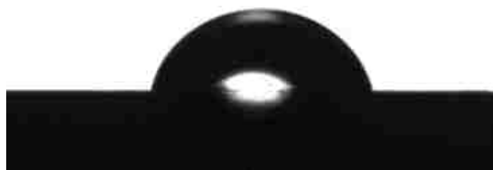
Figure 2.13: Water droplet on a plain Al 6061 surface; average contact angle: 81 °
