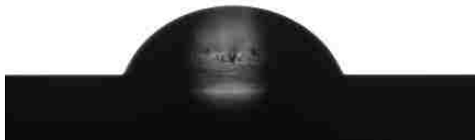
Figure 2.14: Water droplet on TiO 2 coated Al 6061 with NeverWet; average contact angle: 65 °
