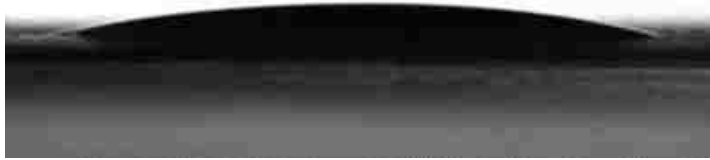
Figure 2.15: Water droplet on a TiO 2 coated Al 6061 surface; average contact angle: 15 °
