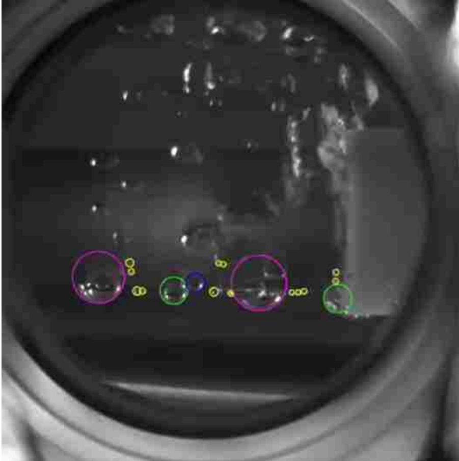
Figure 3.6: Image of bubble detection processed by MATLAB based on the CHT
