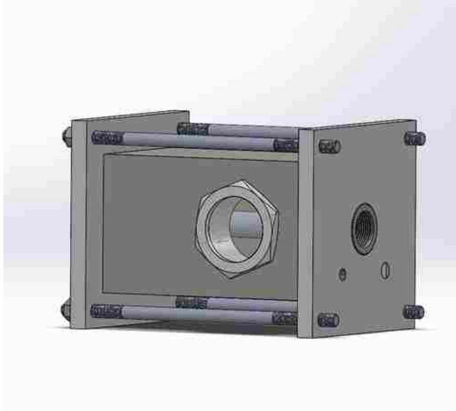
Figure 2.2: CAD of the boiling chamber housing and PTFE plates
