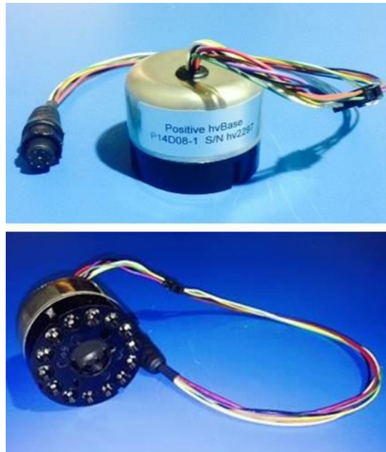
Figure 6: High Voltage Base
