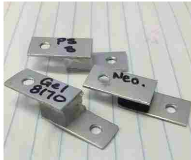
Figure 5: Samples glued to aluminum sheet metal for testing.
