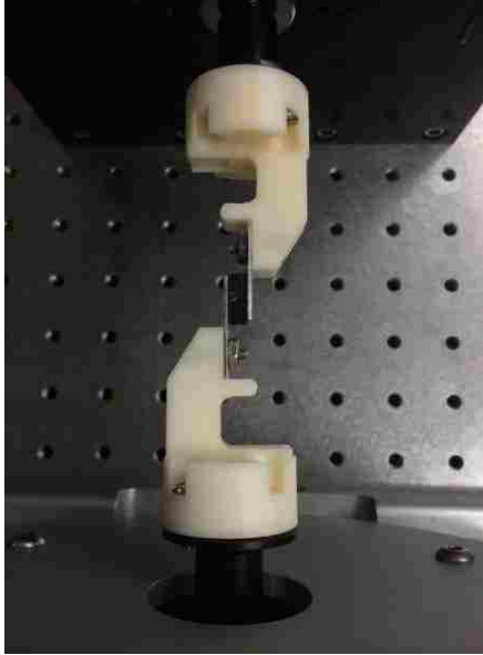
Figure 4: MRE sample being tested for shear modulus in DMA.
