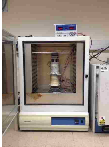
Figure 2: Set up for curing the MRE in magnetic field and heat.
