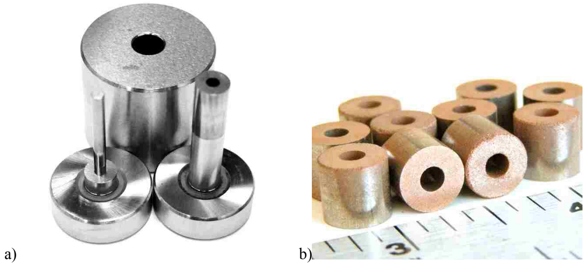
Figure 3. 4: (a) Die and (b) metal hydride pellets prepared for H 2 storage
