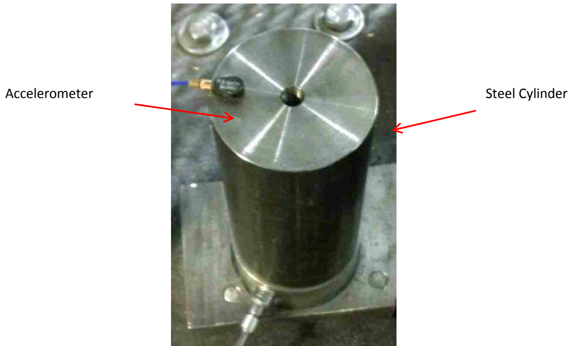
Figure G.3: Steel Cylinder with Accelerometer
