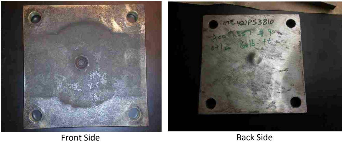
Figure 3.30: Typical 1/2" A36 Plate Damage
