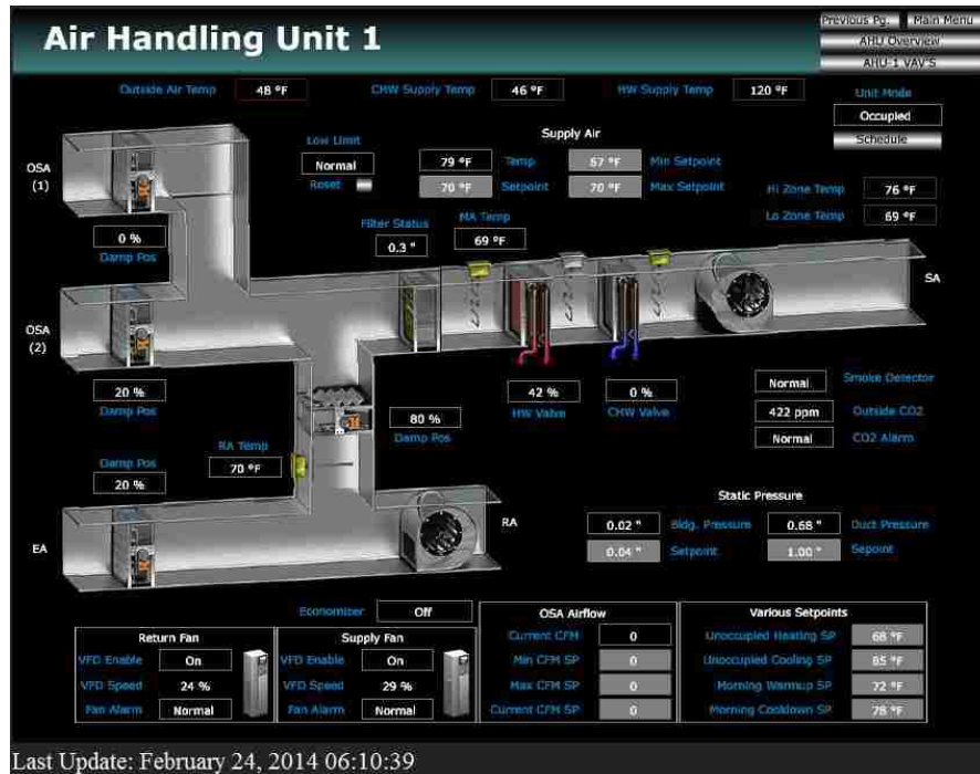
Figure 35. BMS AHU-1 Sample Page.
