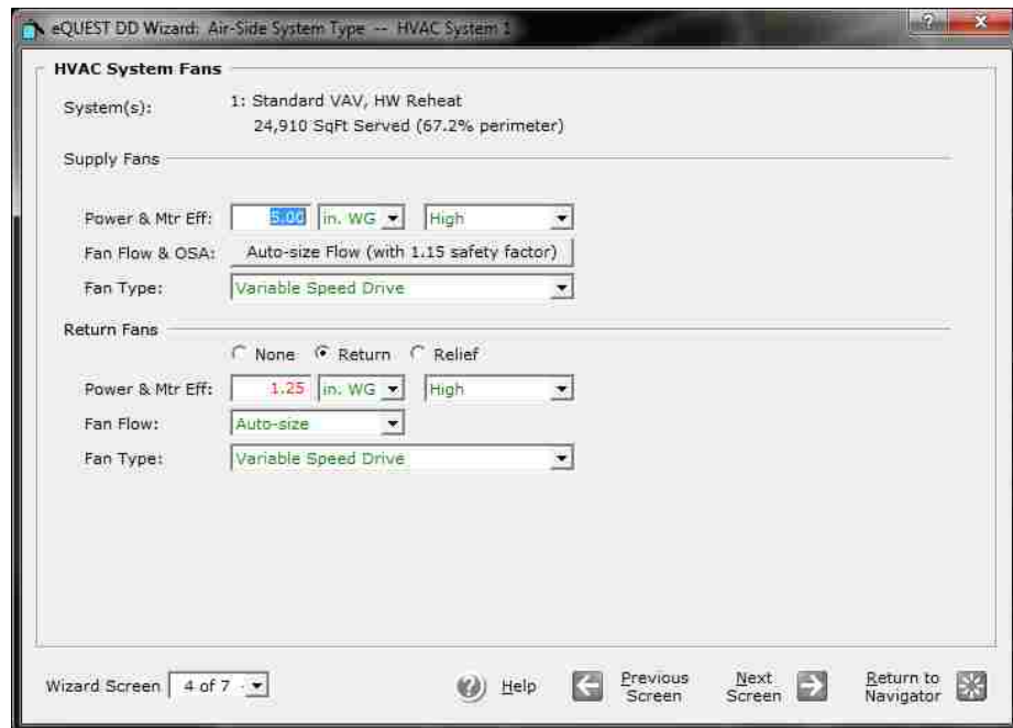
Figure 50. eQUEST Proposed HVAC Fan Definition.
