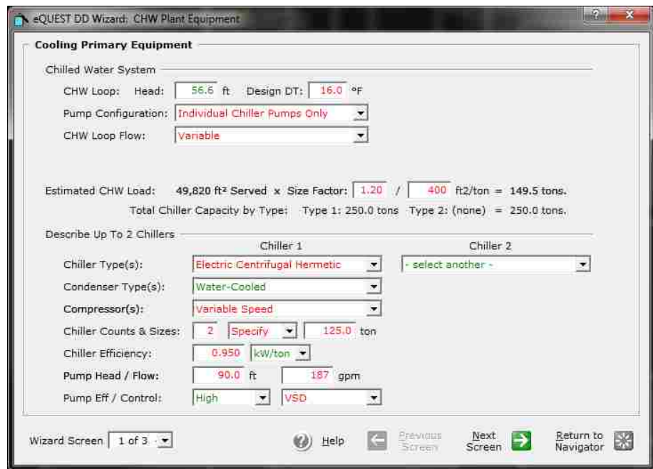
Figure 52. eQUEST Proposed HVAC Cooling Equipment Definition.
