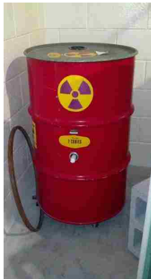
Figure 27 - Plutonium-Beryllium (Pu-Be) Source in the Nuclear Measurements Laboratory at UNLV
