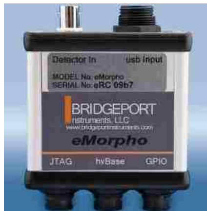
Figure 24 - eMorpho Data Acquisition Device from BPI [57]
