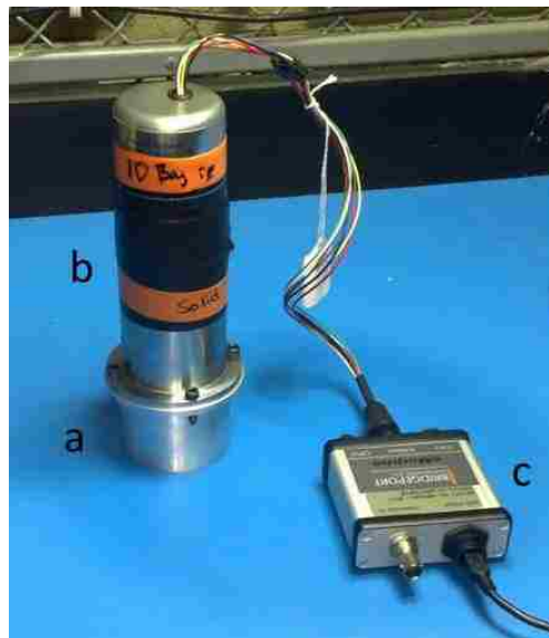
Figure 26 - Plastic Scintillator Detector: (a) the Scintillator Enclosure, (b) the PMT Enclosure, and the (c) eMorpho Hardware
