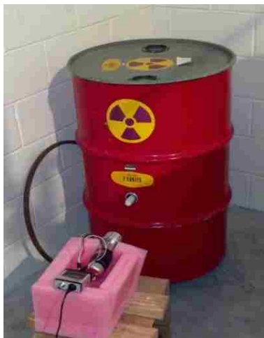
Figure 29 - Single Detector Experiment with Pu-Be Source
