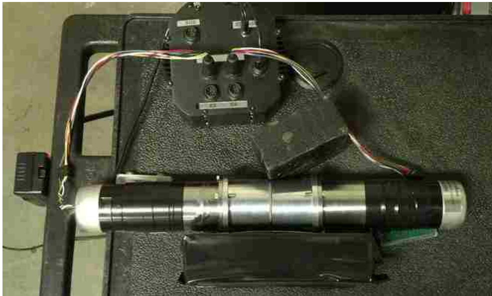
Figure 31 - Time Correlated Measurement using Two Detectors and ^{60}\text{Co} Source
