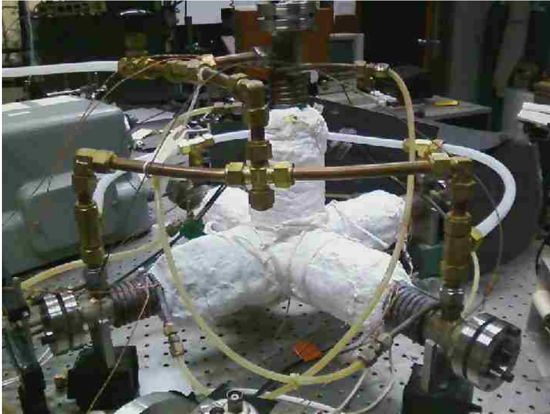
Figure 4.2: A photograph of the heat pipe oven loaded with sodium and potassium for this work. Each arm of the heat pipe is wrapped by a “clam-shell” heater and insulation. Underneath the heaters, there is a total of twelve thermocouple wires. The ends of each arm are capped with BK7 windows held in place by a stainless steel flange. The outer end of each arm is cooled by liquid water carried by copper tubing wrapped around each end. Plastic and copper tubing carries the buffer gas, which makes a whole circuit around the heat pipe oven.
