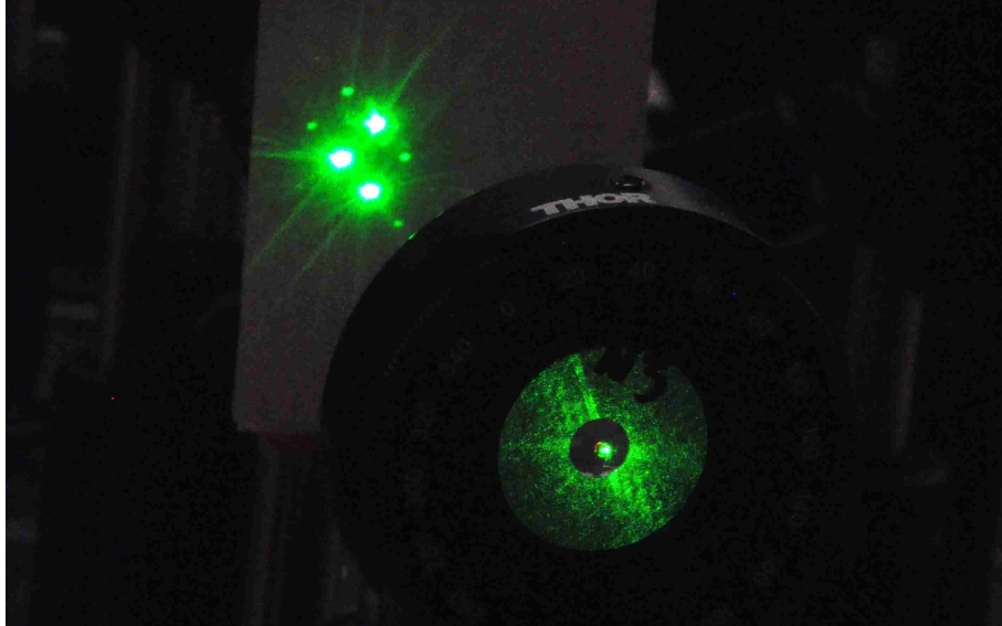
Figure 5.5: Mounted rubrene sample in foreground where the beams meet, and a screen in the background where the transmitted and diffracted beams, in the characteristic formation, are seen for delay time t = 50 ps.
