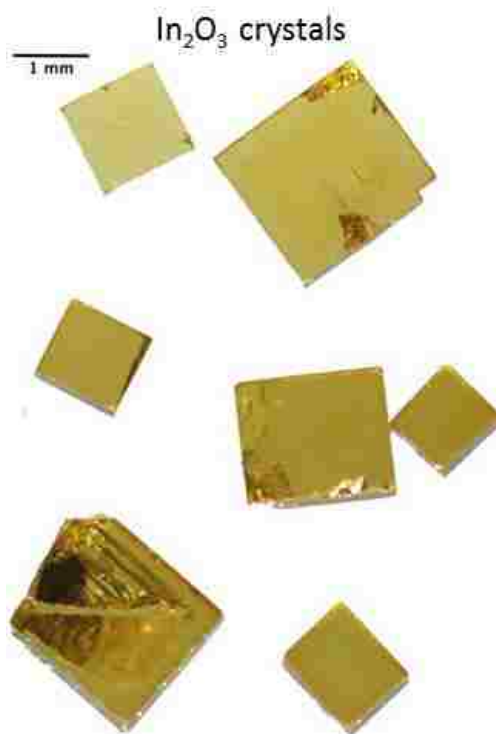
Figure 2.3: In 2 O 3 bulk single crystals grown in an air ambient by the flux method at the Oak Ridge National Laboratory (ORNL) by Dr. Lynn Boatner. These crystals were pale yellow in color.
