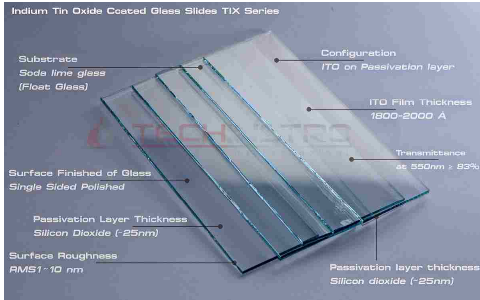
Figure 1.1: Indium Tin Oxide coated glass slides TIX series by TECHINSTRO Co. Specified ITO Sheet resistivity \leq 10 \text{ ohms/sq} ; Transmittance at 550 \text{ nm} \geq 83 \% . http://techinstro.blogspot.com/2014/07/indium-tin-oxide-coated-glass-slides.html .
