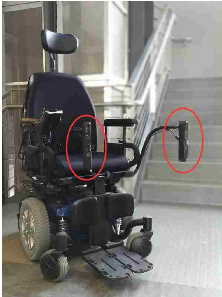
Figure 5.1: CoPilot integrated into an Quantum Q6 Edge EPW. The Primesense Carmine 1.09 sensors are circled in red.
