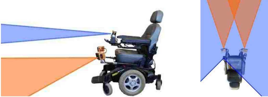
Figure 6.8: The SWS prototype with the fields of view of the actuated LIDAR (blue) and each 3D camera (orange) highlighted. (Left) A profile view and (Right) a top down view of the respective sensors’ fields of view.
