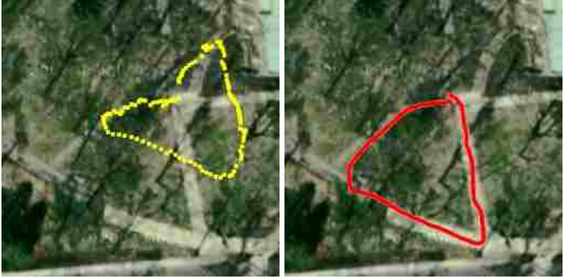
Figure 6.1: A demonstration of the ineffectiveness of GPS as method of sidewalk level localization. (Left) The GPS signal is overlaid on satellite imagery while driving around the triangular-shaped path. (Right) The path derived from SLAM using trees as landmarks.
