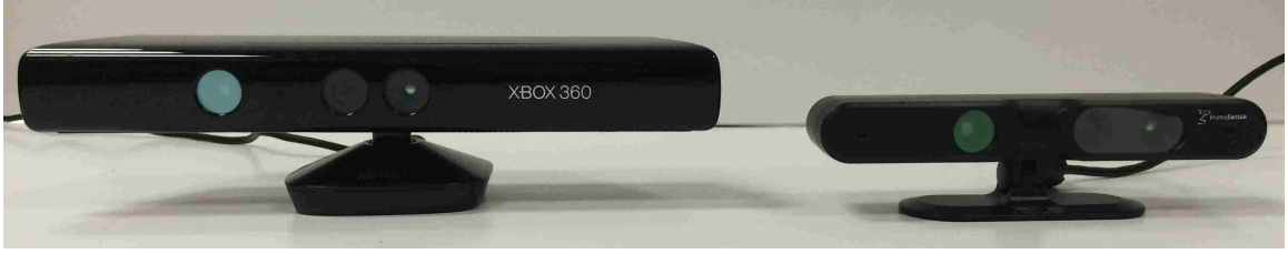
Figure 2.2: Examples of structured light based sensors. (Left) The Microsoft Kinect. (Right) The Primesense Carmine 1.09.
