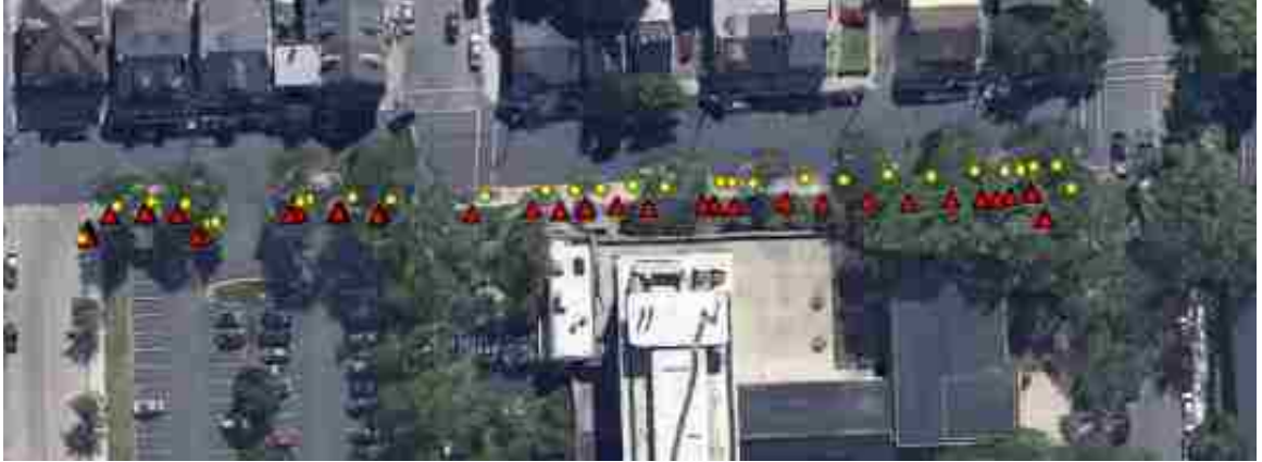
Figure 6.7: A comparison of an initial landmark map to the refined map. The trike started on the left with an acceptable GPS position estimate and traveled to the right up a grade of approximately 8.5%. The red triangles indicate the landmarks in M_{v1} and the yellow circles indicate the landmarks in M_{v2} . A landmark at each corner was tagged with satellite imagery positional information to act as known correspondences.
