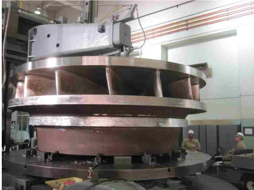
Figure 20: Turning runner on the Cincinnati for final seal ring clearances [2].
