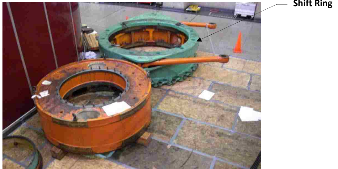
Figure 33: Wicket Gate Servo Motor Arm and Shift Ring Mechanism [2].
