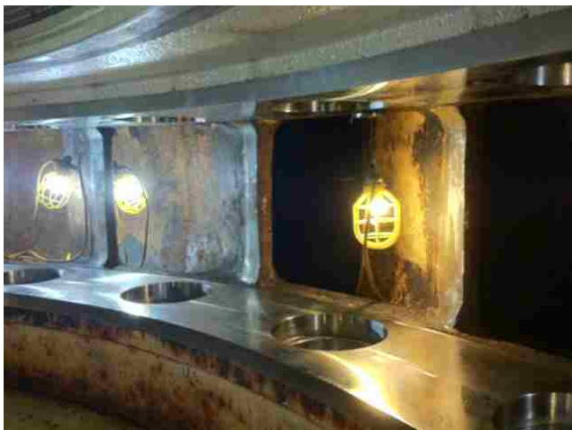
Figure 22: Refurbished Nitronic 60 wear plates [2].
