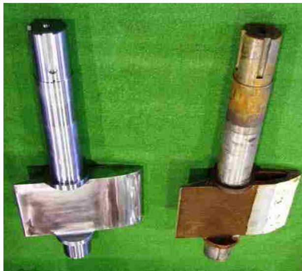
Figure 15: New Stainless Steel Wicket Gate (left) vs. Old Cast Steel Wicket Gate (right) [2].
