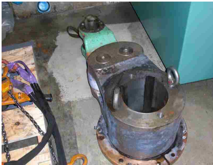
Figure 34: Wicket Gate Linkage Mechanism [2].
