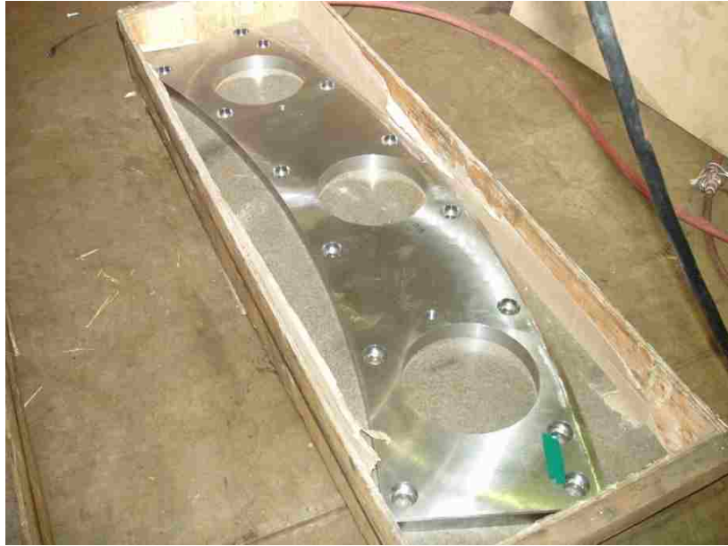
Figure 10: Wear plate ready for bolting above and below wicket gates [2].
