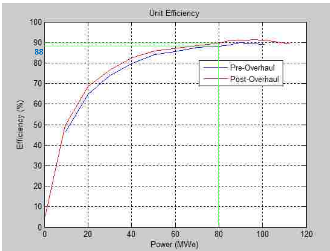
Figure 41: MATLAB ® plot of Unit Efficiency – Pre-Overhaul vs. Post-Overhaul Data.
