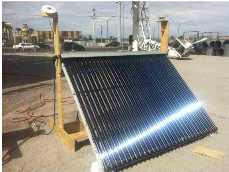
Figure 29. Experiment 2: SolarUS SL-30 Evacuated Tube Collector.
