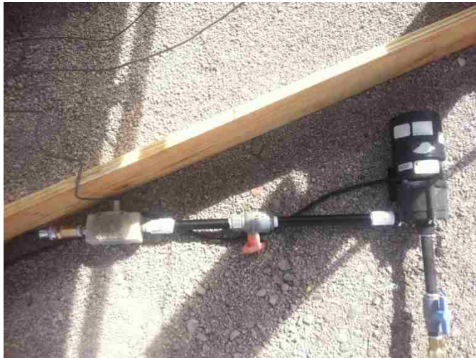
a) b) Figure 31. Experiment 2: System components. a) Pump and flow meter in series b) flow meter operating at about 0.7 gallons per minute.
