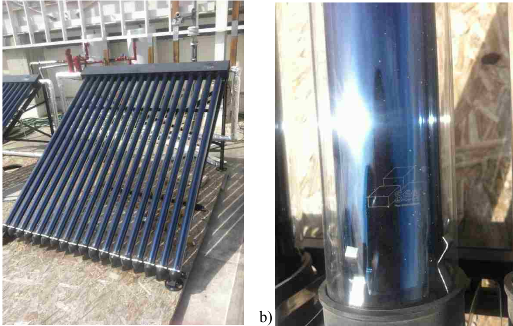
Figure 28. Experiment 1: SEA Evacuated Tube Collector – Set of 18 b) Vacuum tube close-up.
