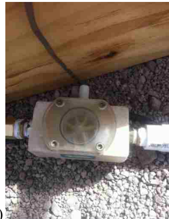
a) b) Figure 31. Experiment 2: System components. a) Pump and flow meter in series b) flow meter operating at about 0.7 gallons per minute.
