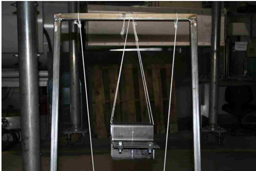
Figure 18: Hanging Mass Structure for Unconstrained Bolted Hat Structure Experiment
