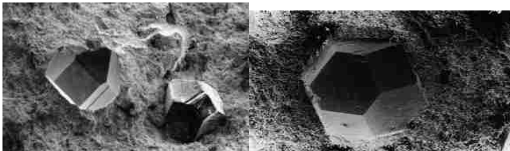
Figure 1.7: Scanning electron microscope (SEM) image of a diamond and metal matrix [22][23]
