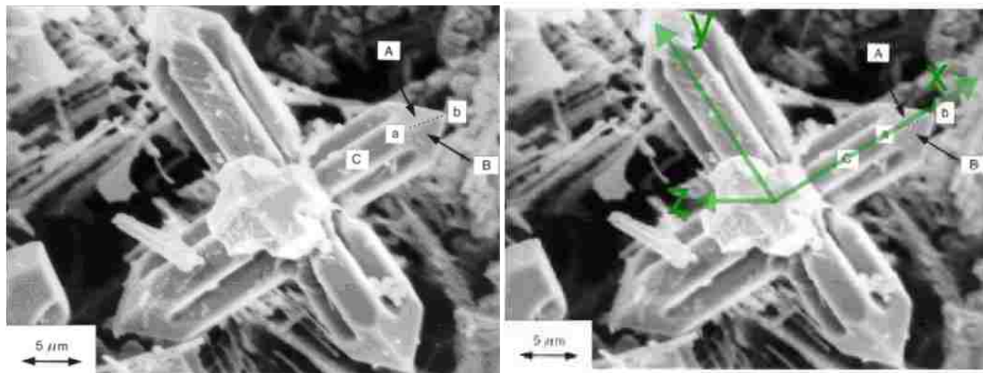
Figure 3.3: Scanning electron microscope figure of niobium carbide dendrite [55]
