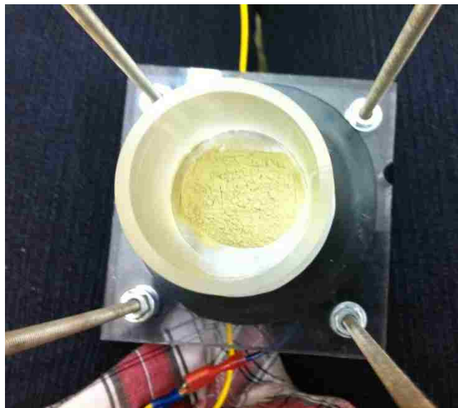
Figure 4.7: Diamond powder covered by hollow cylinder
