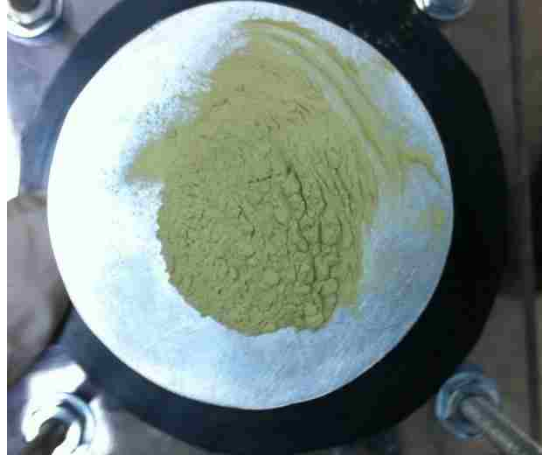
Figure 4.6: Diamond powder on cathode plate
