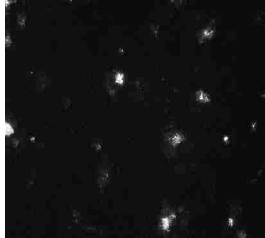
Figure 3.17: Optical image of pad showing contact points at 50 torr
