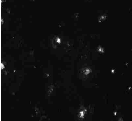
Figure 3.16: Optical image of pad showing contact points at 30 torr
