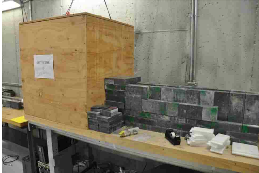
Figure 3.8 HPGe detector and shielding at IAC
