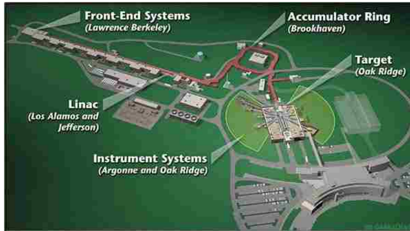
Figure 4.1: Layout of Spallation Neutron Source at Oak Ridge National Laboratory in Tennessee, USA.[2]
