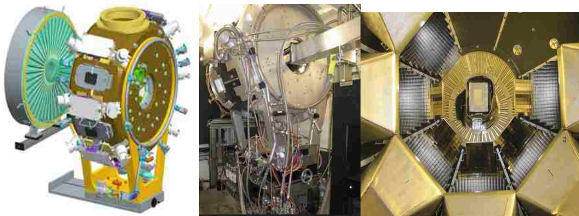
Figure 4.3:VISION instrument : Outside view of the spectrometer chassis, facing upstream (left), real working spectrometer with beam stop (middle), and inside view of the upstream double-focusing crystal array analyzers and corresponding beryllium filter assemblies (right).[3]
