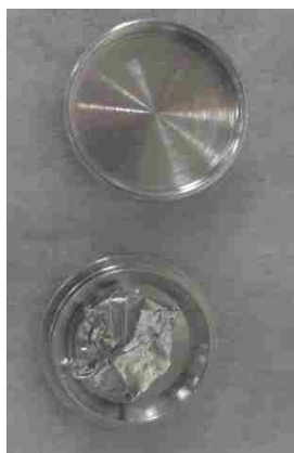
Figure 29. Example of a target prepared to irradiation at Flattop (ruler is in cm).
