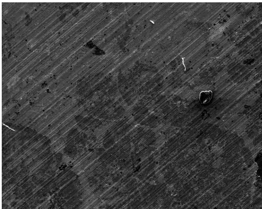
Figure 23. Optical image (top) and SEM image (bottom) of the 2:1 KBr:UO 2 pellet with scale bars.
