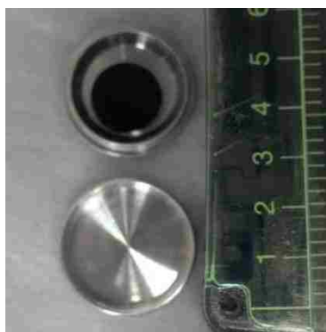
Figure 29. Example of a target prepared to irradiation at Flattop (ruler is in cm).
