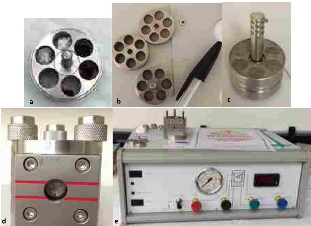
Figure 64. This series of images shows a sample being prepared for critical point drying. A) The basket that holds up to six samples. B) The three parts of the basket compared to a pen cap. C) The fully assembled basket. D) The chamber where the basket sits during the drying. The window shows the level of the CO 2 in the chamber – the meniscus should be between the two red lines in order for the process to work. E) The benchtop critical point dryer. The chamber is located on the top left of the instrument.
