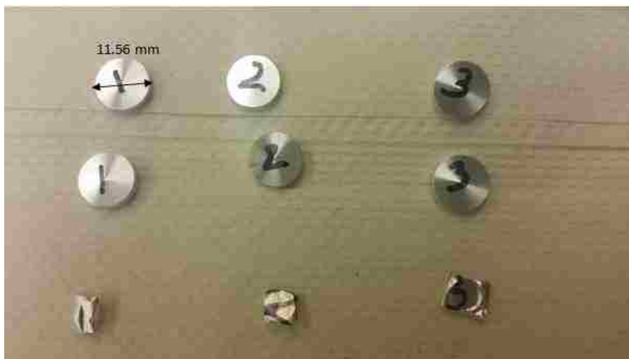
Figure 30. Examples of sample holders labeled for an irradiation. The foil-wrapped targets at the bottom of the image were placed into their respective sample holders.
