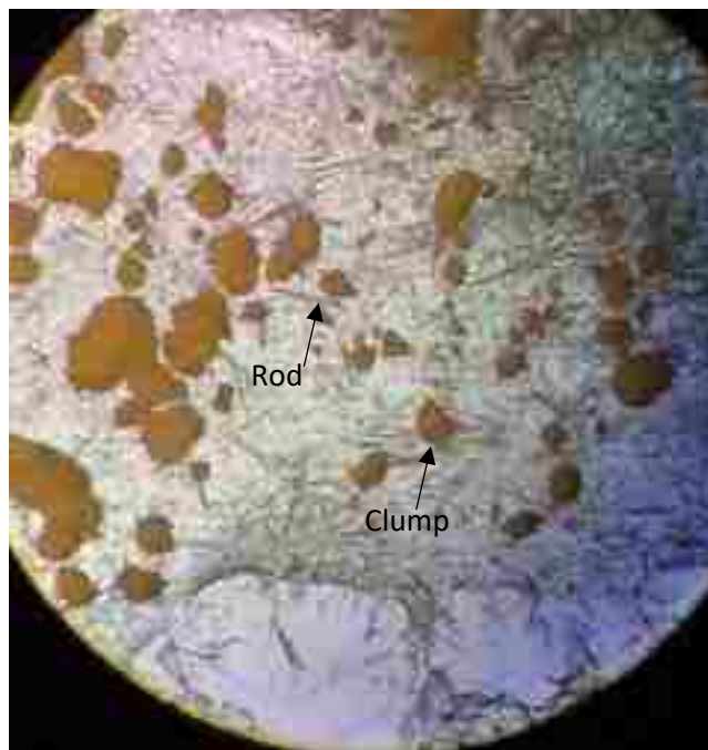
Figure 44. Microscope image of the material showing both crystalline clumps and rod-shaped crystals.
