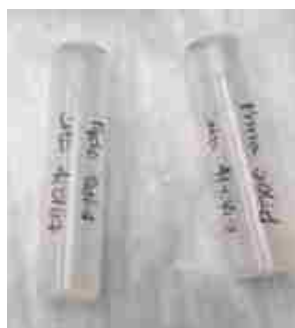
Figure 57. 5 mL plastic scintillation vials like these were used to hold the samples as they were counted.
