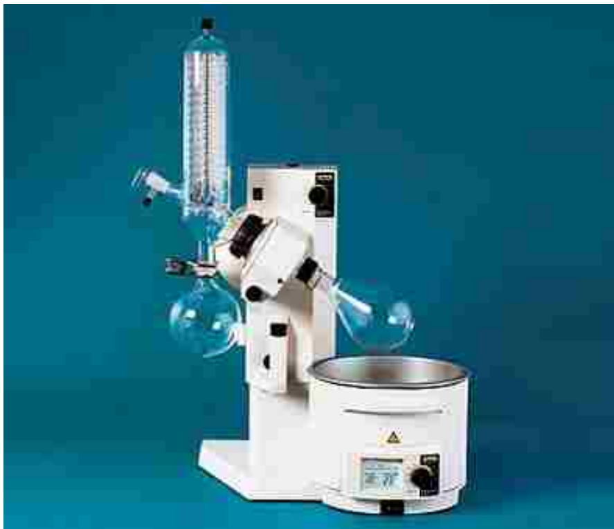
Figure 1-3 Typical Rotovap Evaporation Apparatus
