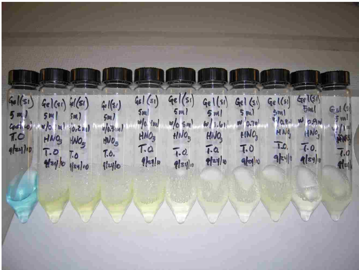
Figure 3-17. Hydrogel Polymer with Varying \text{HNO}_3 (The control gel is on the left, acid concentration increases toward the right) – no scale.
