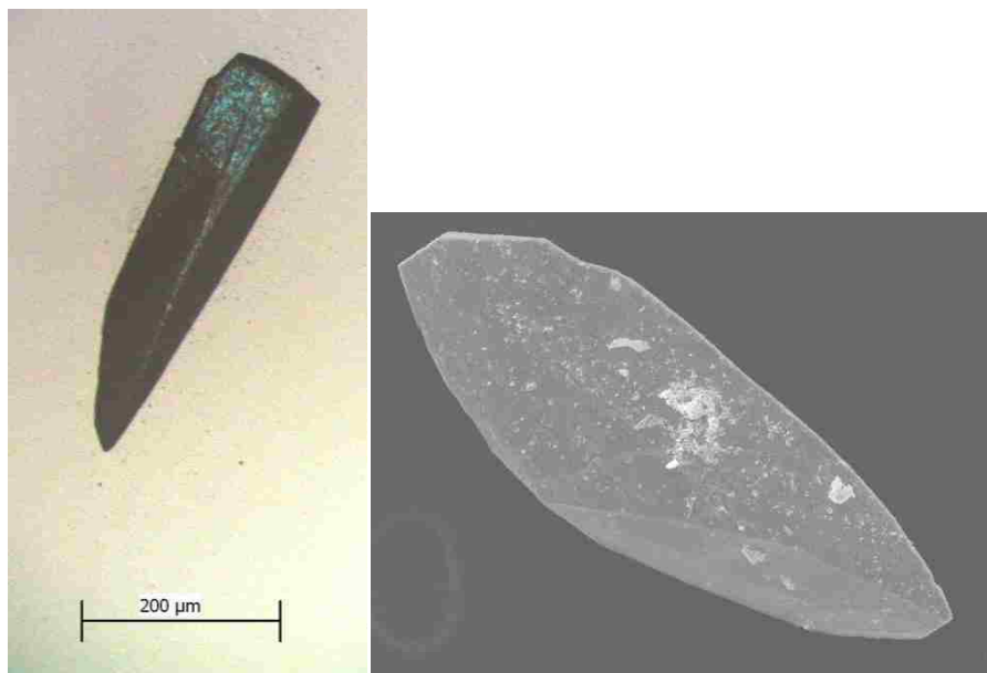
Figure 3.12. Left: Optical microscopy image of a single rail spike crystal of \text{Na}\{[\text{Tc}_6\text{Br}_{12}]_2\text{Br}\} . Right: Scanning electron microscopy (SEM) image of a single rail spike crystal of \text{Na}\{[\text{Tc}_6\text{Br}_{12}]_2\text{Br}\} at x500 magnification.
