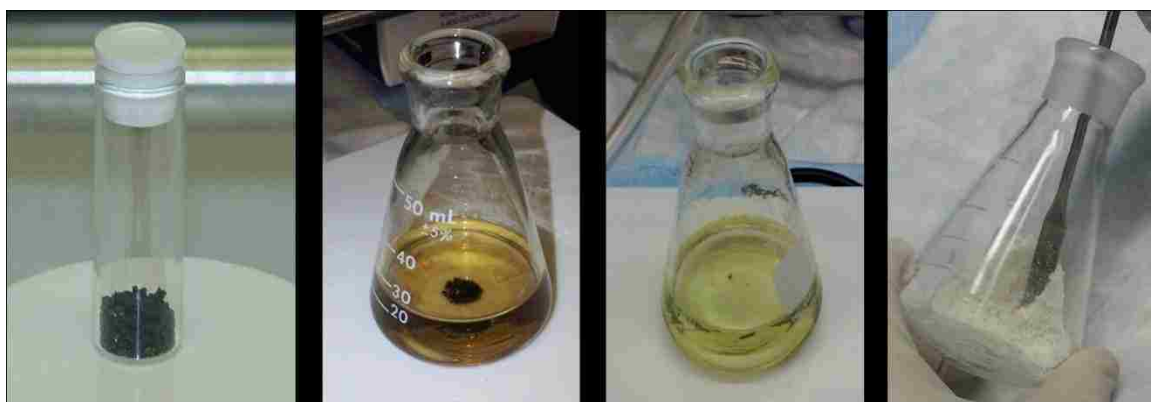
Figure 2.1. Purification of \text{NH}_4\text{TcO}_4 starting with the impure material from ORNL (left) to purified \text{NH}_4\text{TcO}_4 (right).
