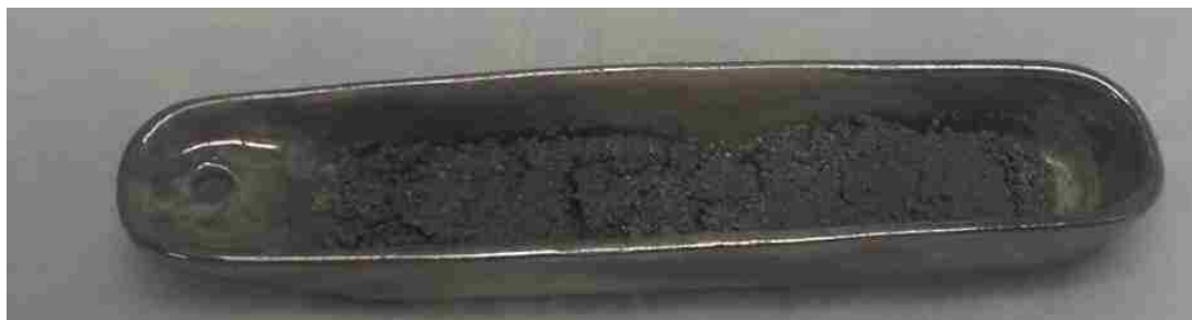
Figure 2.2. Technetium metal obtained after the decomposition of \text{NH}_4\text{TcO}_4 under \text{H}_2(\text{g}) at 750\text{ }^\circ\text{C} .
