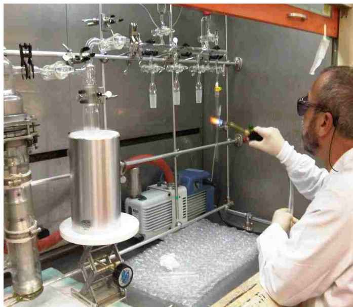
Figure 2.8. Sealing a Pyrex tube under vacuum on a high vacuum Schlenk line.
