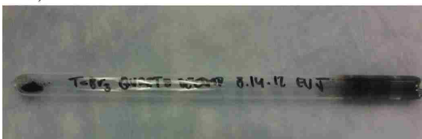
Figure 4.19. Resulting tubes from the thermal decomposition of \text{TcBr}_3 in a) Pyrex yielding rail spike crystals adjacent to the powder (black circle) and needle crystals at the end of the tube and in b) quartz with only sublimed needle-shaped crystals.
