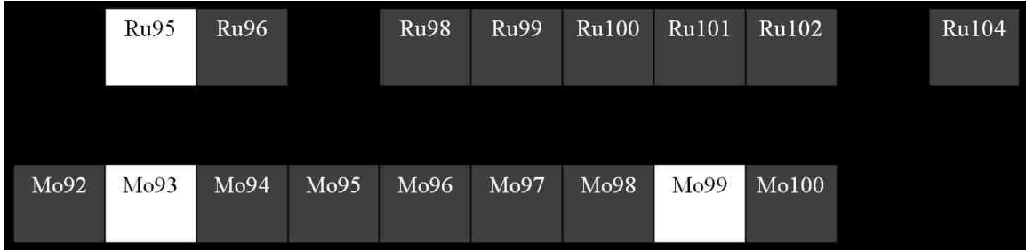
Figure 2. An excerpt from the Chart of the Nuclides of isotopes of Mo ( Z = 42 ) to Ru ( Z = 44 ) illustrating the abundance of stable isotopes of Mo and Ru surrounding technetium. Stable isotopes are in black [1b].
