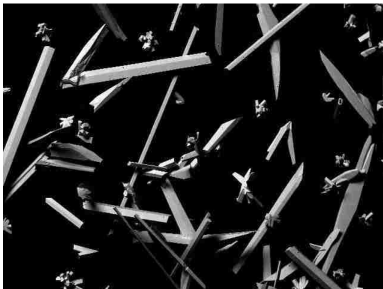
Figure 4.20. SEM image (x35) of TcBr 3 single crystals as individual and clusters of needles ranging in size from 100 μm to 2 mm.
