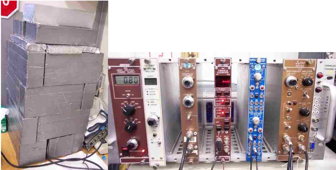
Figure 14. NaI well detector setup
