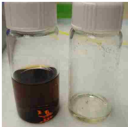
Figure 3.5. Mother liquor solution removed from original vial after two days, revealing crystals of Tc_2(O_2CCH_3)_3Cl_2(H_2O)_2 \cdot H_2O seen on the bottom and sides of the empty vial. The clear liquid in the bottom of the vial on the right is paratone oil used to obtain single crystals for XRD.
