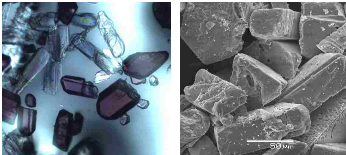
Figure 4.4. Optical microscope view (right) of single crystals Tc_2(O_2CCH_3)_4(\mu-O_2CCH_3) , and SEM-image magnification x500 in scanning electron mode(left).
