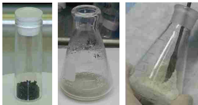
Figure 2.1. \text{NH}_4\text{TcO}_4 from Oak Ridge (left), dissolution and purification of bought pertechnetate (middle) and white precipitate \text{KTcO}_4 (right).
