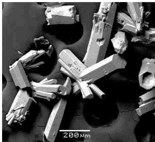
Figure 3.3. Leica optical microscope images of Tc_2(O_2CCH_3)_4Br_2 on the right and SEM image magnification \times 90 in back scattering mode on the left.
