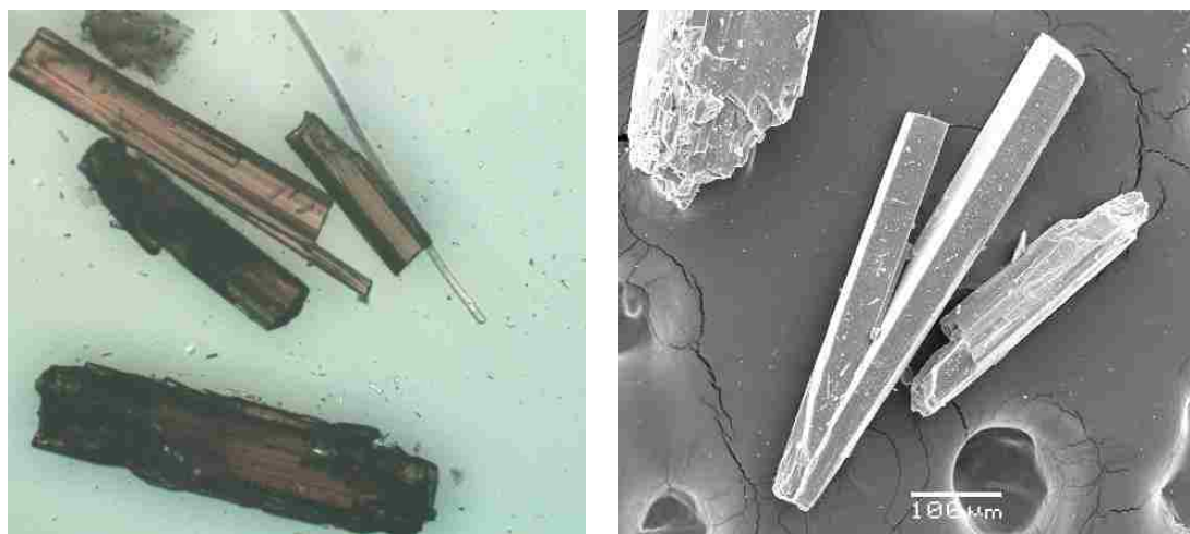
Figure 4.6. Optical microscope view (right) of single crystals \text{Tc}_2(\text{O}_2\text{CCH}_2\text{CH}_3)_4(\mu\text{-O}_2\text{CCH}_2\text{CH}_3) , and SEM-image magnification \times 150 in scanning electron mode (left).
