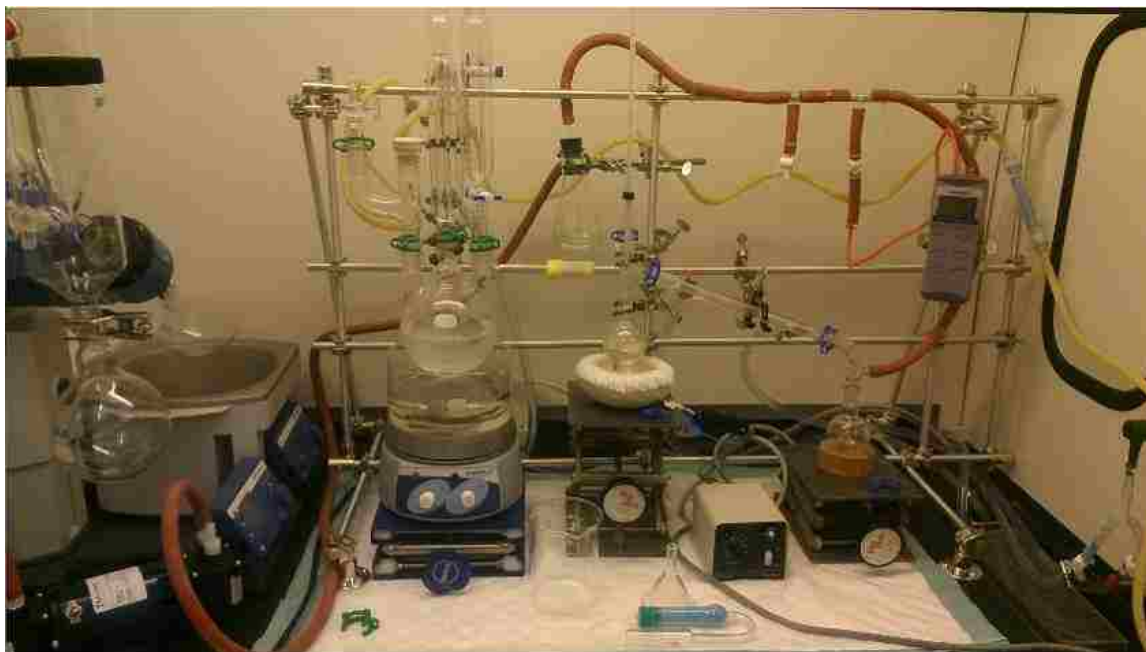
Figure 31. Experimental set up showing reaction vessel, rotary evaporator and distillation apparatus.
