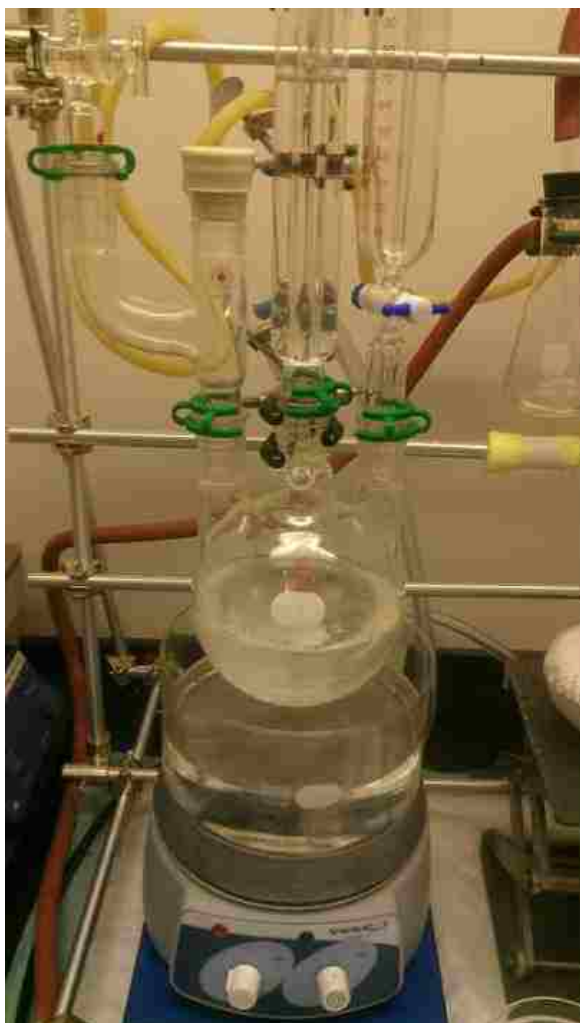
Figure 32. Addition of Na metal under nitrogen atmosphere to ethanol.
