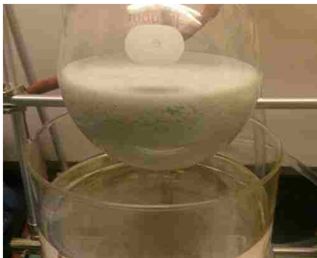
Figure 34. 2,2'-[Thiobis(2,1-ethanediythio)]bis(ethanol) product with NaCl prior to dissolving in hot acetone and filtering.
