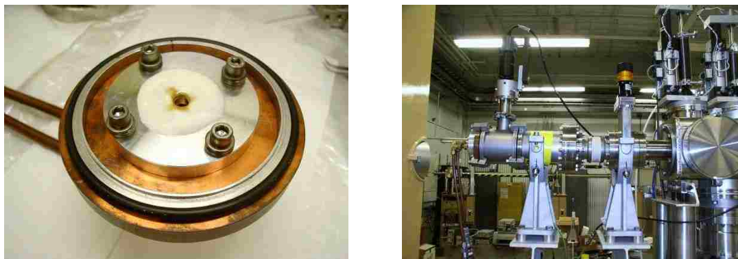
Figure 42. CAMS target chamber for irradiations of stable metal foils: copper cooling block with aluminum clamp to hold foil stack in place (left) and the irradiation chamber as installed at the CAMS beamline (right).
