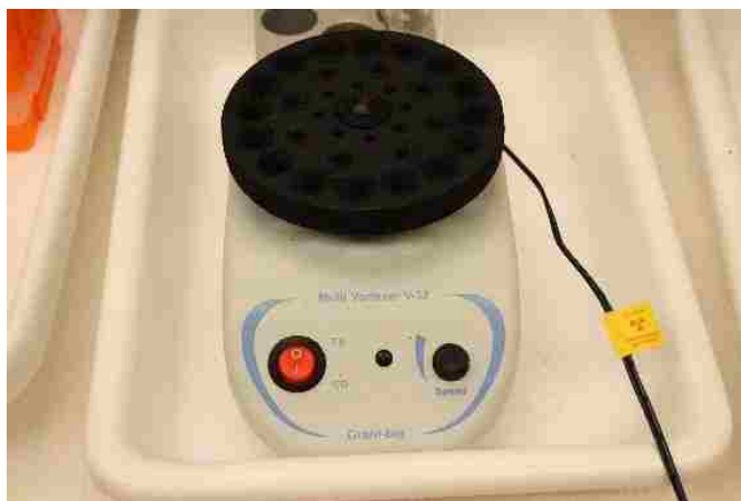
Figure 22. Grant-bio Multi-tube Vortex Mixer.
