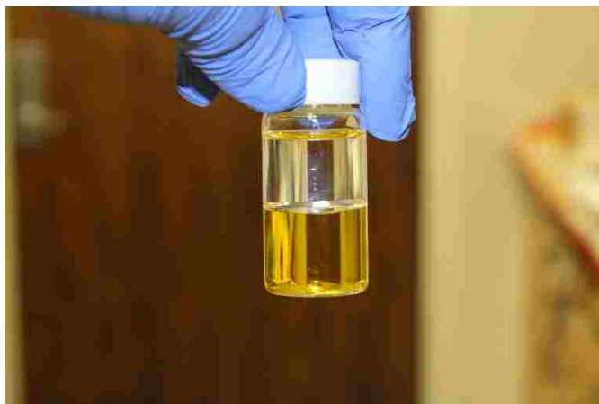
Figure 18. Diagram of SX where a solute would be distributed between two immiscible solvents. In this example an organic phase, such as toluene, is on the top, and an aqueous phase, such as hydrochloric acid, is on the bottom (color added for clarity).
