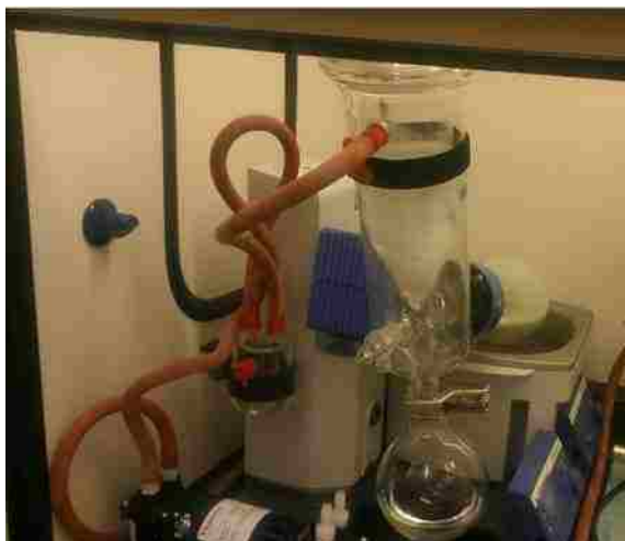
Figure 36. 1,1'-[Thiobis(2,1-ethanediylthio)]bis[2-chloroethane] product during rotary evaporation.
