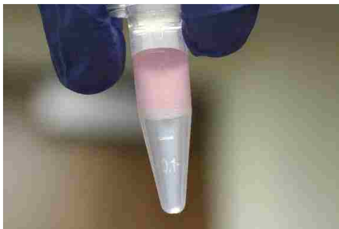
Figure 26. Organic phase (dichloromethane) and aqueous phase in VWR 1.5-mL high spin centrifuge tube (pink color of aqueous phase added for visual purposes only).
