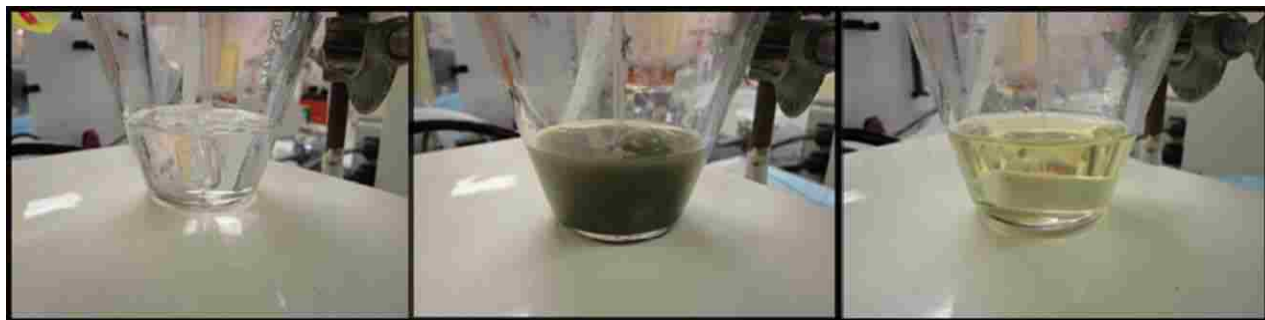
Figure 31. The IL before (left), during (middle), and after (right) dissolution of U_3O_8
