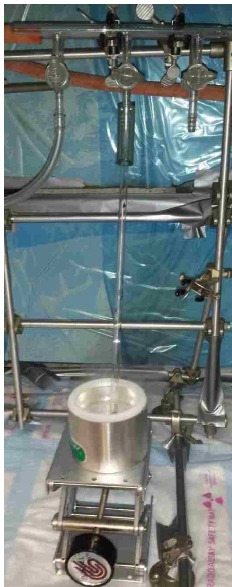
Figure 2.4. Experimental set-up used for the condensation of liquid O 2 into a glass tube.
