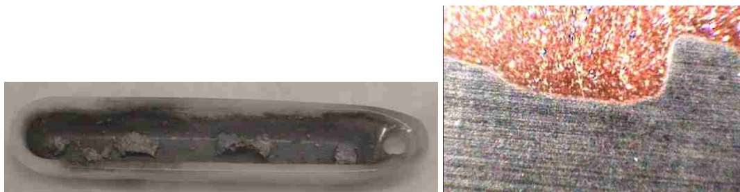
Figure 1.10. Tc metal obtained after hydrogen reduction of \text{NH}_4\text{TcO}_4 (left) and electroreduction of \text{TcO}_4^- in \text{H}_2\text{SO}_4 on a Cu electrode (right).
