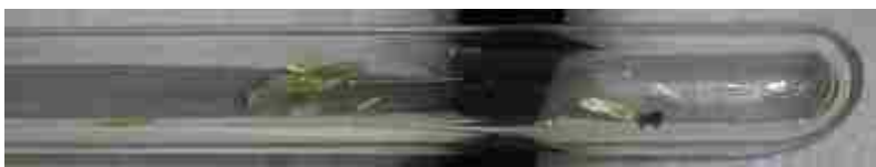
Figure 4.1 \text{Tc}_2\text{O}_7 crystals in sealed tube obtained after the oxidation of \text{TcO}_2 by \text{O}_2 at 450\text{ }^\circ\text{C} .
