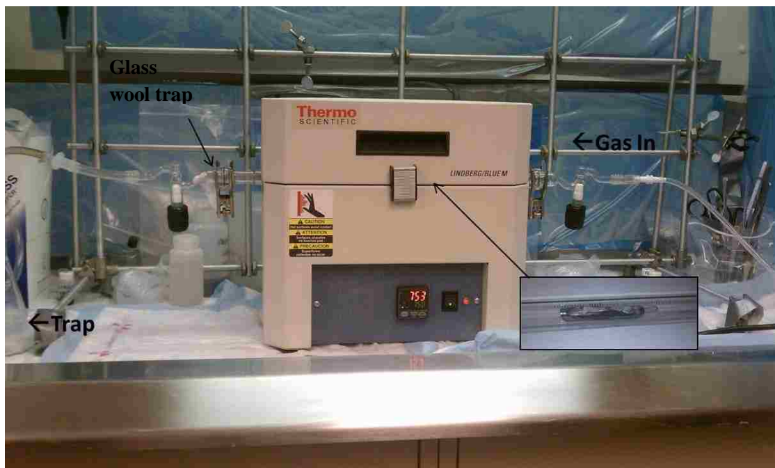
Figure 2.6. Flowing glass setup used for the vitrification of Tc in glass.
