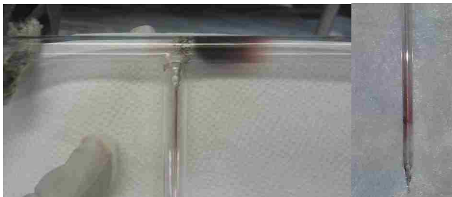
Figure 5.3. Left: red film and \text{Tc}_2\text{O}_7 produced during the oxidation of \text{TcO}_2 with \text{O}_2/\text{H}_2\text{O} . Right: the protective tubing has been removed.
