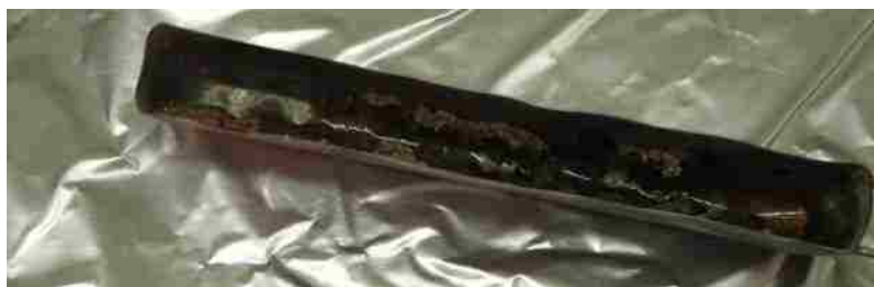
Figure 2.5. Glass that was vitrified at 900 °C in a platinum boat.
