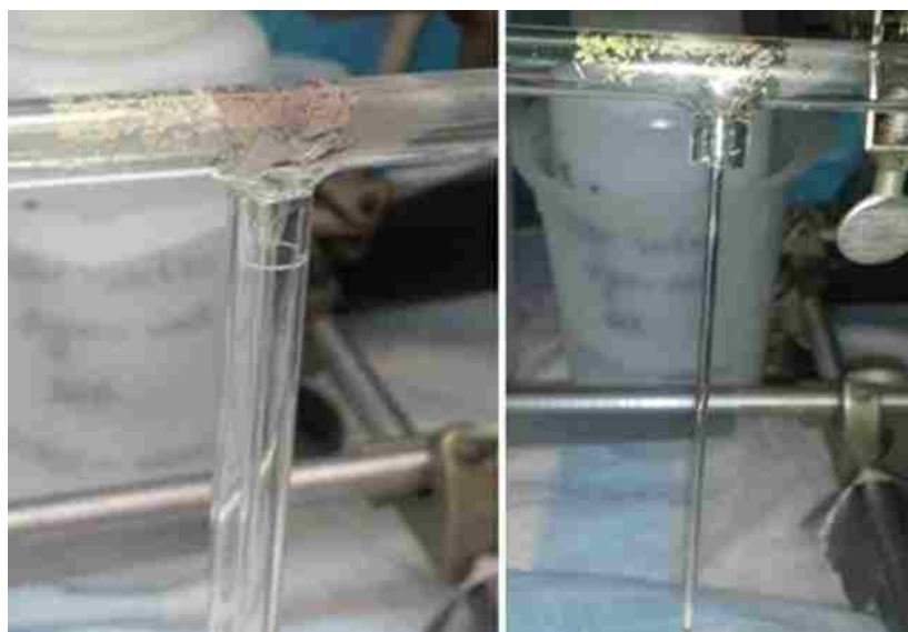
Figure 4.4 (Left) Crystals of \text{Tc}_2\text{O}_7 with a red film over the tube where \text{Tc}_2\text{O}_7 was collected. (Right) The protective tubing has been removed leaving only the 1.96 mm OD tube with \text{Tc}_2\text{O}_7 at the bottom.
