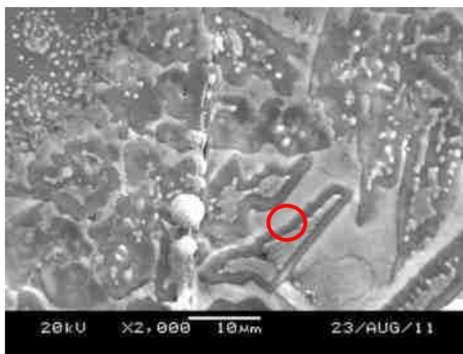
Figure 3.5. SEM image of glass synthesized in air (x2000) at 1100 °C. The red circle (region C) indicates where the EDX measurement was performed.
